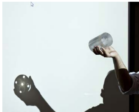
Fig. 7 A CT phantom is used to demonstrate the phenomenon of x-ray scatter and its impact on image contrast.
