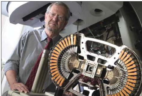
Wolfgang Schlegel with the „Micro-Multi-Leaf Collimator“, which was developed by his group for applications in conformal stereotactic radiotherapy and radiosurgery.
