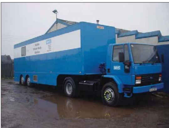
The mobile whole body counter used to measure uptake of radioactivity in the population of UK following the Chernobyl accident. Professor Boddy led the project.
