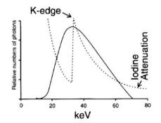
Fig. 11. Iodine Attenuation compared to the effective energy of a 70 kV X-ray Beam Spectrum with 3 mm aluminum total filtration. The effective energy of the x-ray beam spectrum,  $\sim$  30 keV, is well matched to the 33 keV kedge of iodine. This matching increases the radiopacity of an iodine-filled vessel. Reprinted with permission. [83]
