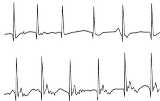
Figure 2. ECG signal collected from patient outside (top) and inside (bottom) an MRI scanner.
