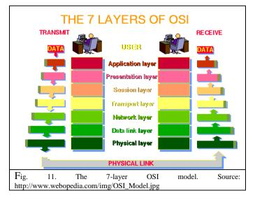
The OSI 7-layer model describes the transmission of messages. In sending a message, each layer (from the highest – the Application – to the lowest – the Physical)
