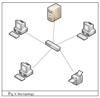
Most small (e.g. home) networks use the star topology. A star network features a central connection point called a "hub node" that may be a network hub, switch or (more likely) a router. Devices typically connect to the hub with Unshielded Twisted Pair (UTP) Ethernet.
