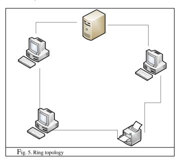
In a ring network, every device has exactly two neighbours for communication purposes. All messages travel through a ring in the same direction (either "clockwise" or "counterclockwise"). A failure in any cable or device breaks the loop and can take down the entire network.
