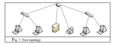
Tree topologies integrate multiple star topologies together onto a bus. In its simplest form, only hub devices connect directly to the tree bus, and each hub functions as the root of a tree of devices. This bus/star hybrid approach supports future expandability of the network much better than a bus (limited in the number of devices due to the broadcast traffic it generates) or a star (limited by the number of hub connection points) alone.
