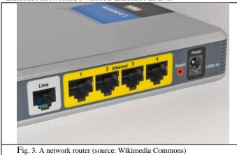
A router forwards data packets along networks. A router is connected to at least two networks and is located at a gateway, the place where two or more networks connect. Routers use headers and forwarding tables to determine the best path for forwarding the packets, and they use protocols such as ICMP (Internet Control Message Protocol) to communicate with each other and configure the best route between any two hosts.
