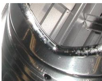
Fig. 10 Foot point craters on a used cathode head after severe vacuum discharge activity (arcing), adapted from [1].
