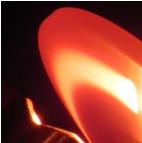
Fig. 5 Thermal picture of a rotating anode in operation. The rectangular focal spot, 10 mm in length and about 1 mm wide, points radially and is located at the right on the anode, trailed by a comet tail of the hot surface of the focal spot track. The X-ray focal spot is located about half a focal spot width further to the right. Some reflected light is visible from the heated electron emitter coil in the cathode at the left. The anode rotated counter clock wise with about 50 Hz. (Adapted from [1].)
