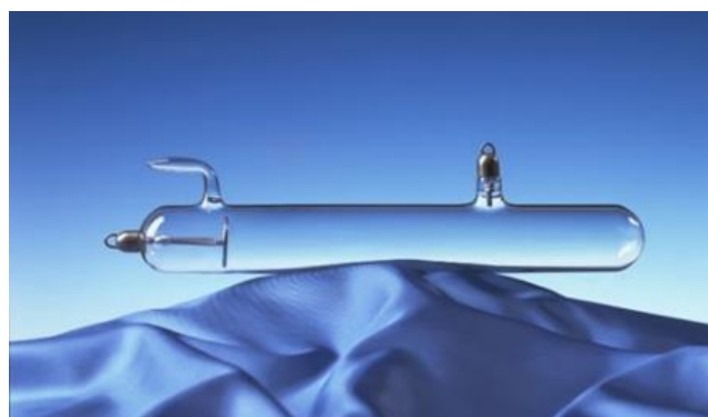
Fig. 1 Replica of an early ion X-ray tube as used by C. W. Roentgen. When the electron collector (short wire, right) is charged positively during the cycle of alternating high-voltage from the inductor and acts as an anode ions generated in the residual gas hit the aluminum slab on the left, the cathode. Cathode rays (electrons) are released, accelerated in the electric field, by-pass the anode wire and hit the glass wall at the right. Greenish fluorescence signals electronic current flow and X-ray generation. Backscattered electrons are collected by the anode wire. Roentgen wrote on Feb. 26 th , 1896: "Namely, I discovered, that X-rays are not only created in glass, but also all other solid bodies (and perhaps even in liquids and gasses)..." (Translated from [2], pg. 56). (Photo courtesy of Philips.)
