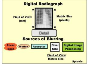
Fig. 6 Pixel size is one of the several sources of blurring in digital radiography. The sources combine to form the total or composite blur that will appear in the image.
