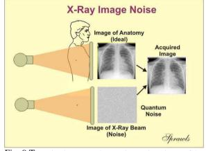
Fig. 9 The noise that appears in x-ray images is an image of the x-ray beam.
