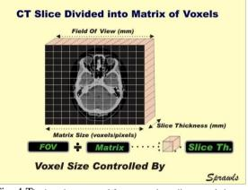
Fig. 4 The imaging protocol factors used to adjust voxel size.
