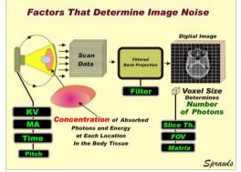
Fig. 11 The adjustable protocol factors that determine noise in CT images.
