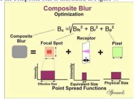
Fig. 7 A general relationship for determining the composite blur value in digital radiography.
