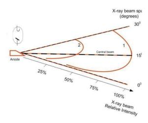
Fig.4 X-ray tube intensity spatial distribution for new X-ray tube (curve 1) and an old one (curve 2). The X-ray intensity is shown in relation to the maximum intensity (100%) at the middle of the central beam of a new X-ray tube. Note also the shifting of the maximum of the intensity from the central beam ( $15^{0}$ ), what leads to significant decrease of the beam intensity at the side of the Anode – i.e. increased Heel effect.
