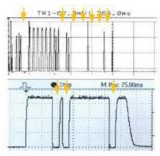
Fig.3 kVp oscillograms of X-ray tubes during arcing (see arrows) -Above: arcing of tube with classical X-ray Generator - some kVp pulses are missing in clusters, as arcing is associated with these (the uneven kVp amplitudes are another sign of micro sparks).
