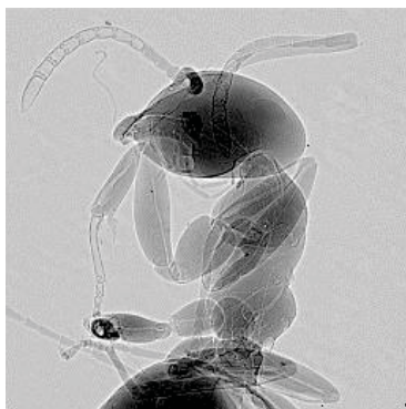
Fig. 10 Phase contrast radiograph of an ant taken at 40 kV, 20 mAs, with a microfocus X-ray tube (5 \mu\text{m} focal spot size) and with a magnification M = 9.1 , R_1 = 68 mm, R_2 = 552 mm (from ref. 21). Important edge enhancement effects are visible, which permit to clearly delineate the silhouette of all low-absorption details of the insect.
