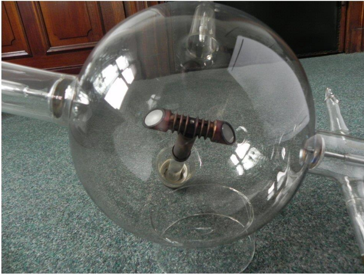
Figure 6 Ion tube for stereoscopic imaging from 1912 after Dr. Fürstennau produced by the H. Bauer GmbH, Jena, Germany or Radiologie GmbH, Berlin, Germany. (Picture taken at the Siemens X-ray tube museum Rudolstadt, Germany.)
