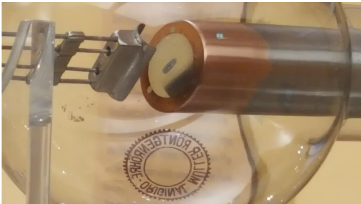
Figure 30 Focusing elements of a stationary anode tube with line focus from C.H.F. Müller, Hamburg, Germany, later Philips. The line focus is mapped in the melting structure on the anode.
