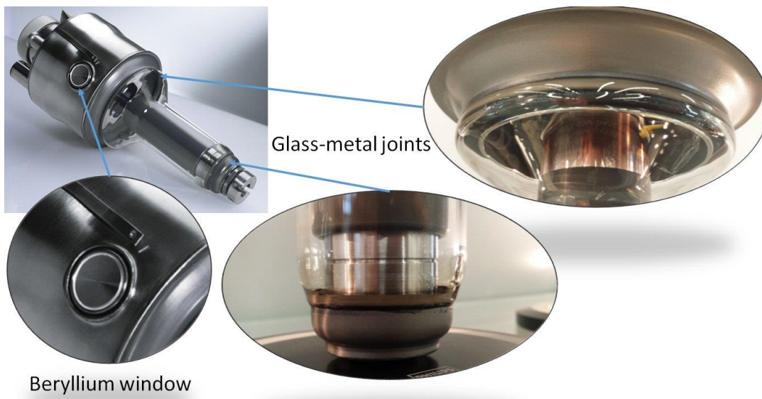
Figure 43 Philips metal center section tube technology with steel frame, alumina coated beryllium X-ray window and glass-metal joints.
