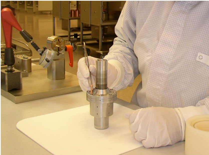
Figure 35 Final assembly of a liquid metal bearing system for the Philips MRC™ 200 angiography tube series.
