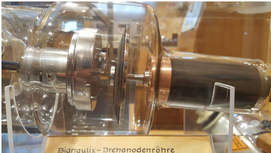
Figure 18 Siemens Biangulix™ tube. Its anode has two separated focal spot tracks with different anode angles. (Picture taken at the Medizinhistorisches Museum Hamburg, Germany, UKE.)
