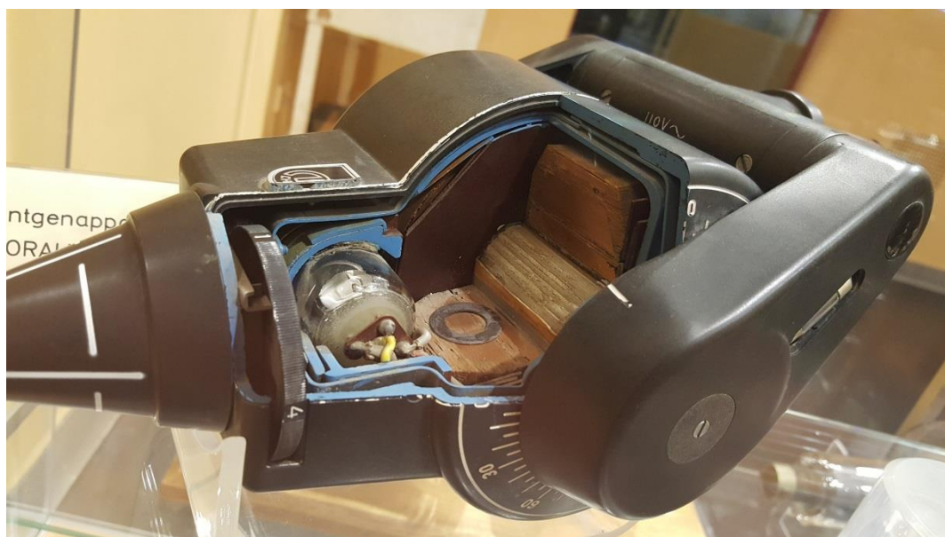
Figure 47 Cut-off picture of a Philips Oralix™ dental tube head. Tube current and focal spot size were stabilized with a Wehnelt electrode and self-controlled resistive biasing. (Picture taken at the Medizinhistorisches Museum Hamburg, Germany, UKE.)
