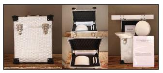
Fig. 2. The U-QA phantom package showing the phantom, user's manual and data analysis software in a travel case.
