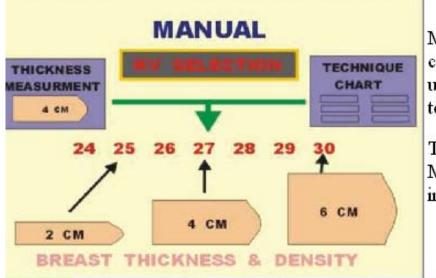
Mammography systems have indicators that display the thickness of the compressed breast. This along with a general assessment of breast density is used to <u>manually</u> select an optimum KV either from experience or an established technique chart.
