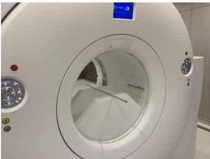
Figure 5 Sensitivity phantom 5 layers of metallic cylinder inserted by polyethylene tube of 700 \pm 20 mm filled with ^{18}\text{F} solution. Acquisitions of 5,4,3,2 and 1 layers at center and 10 offset of FOV
