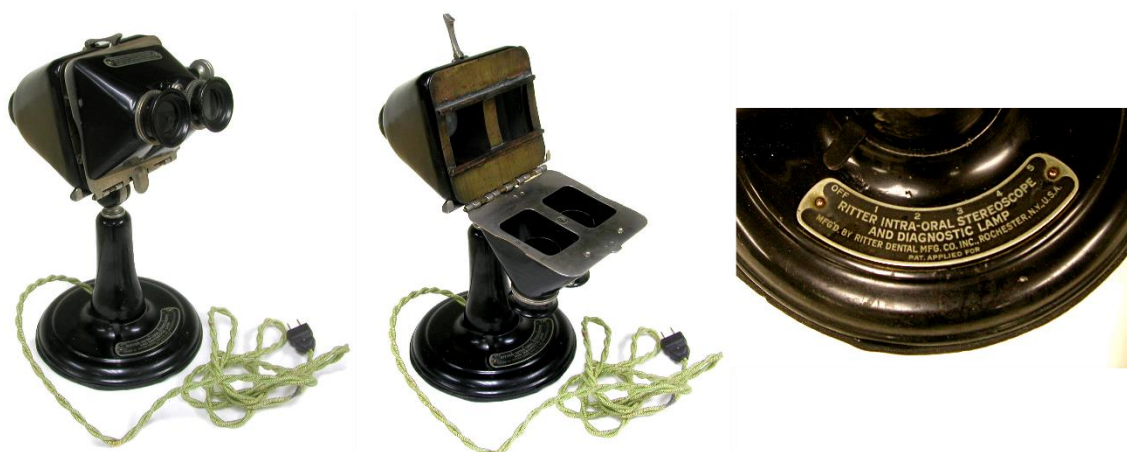
Fig. 13 Ritter intra-oral 'stereoscope and diagnostic lamp' (ca. 1930, pre-patent [41]), used for pseudo-3D diagnosis based on multiple radiographs until at least the 1950s. Pictures and information provided by the Oak Ridge Associated Universities (ORAU) Health Physics Historical Instrumentation Museum Collection under a non-transferable, non-exclusive, limited license [42].
