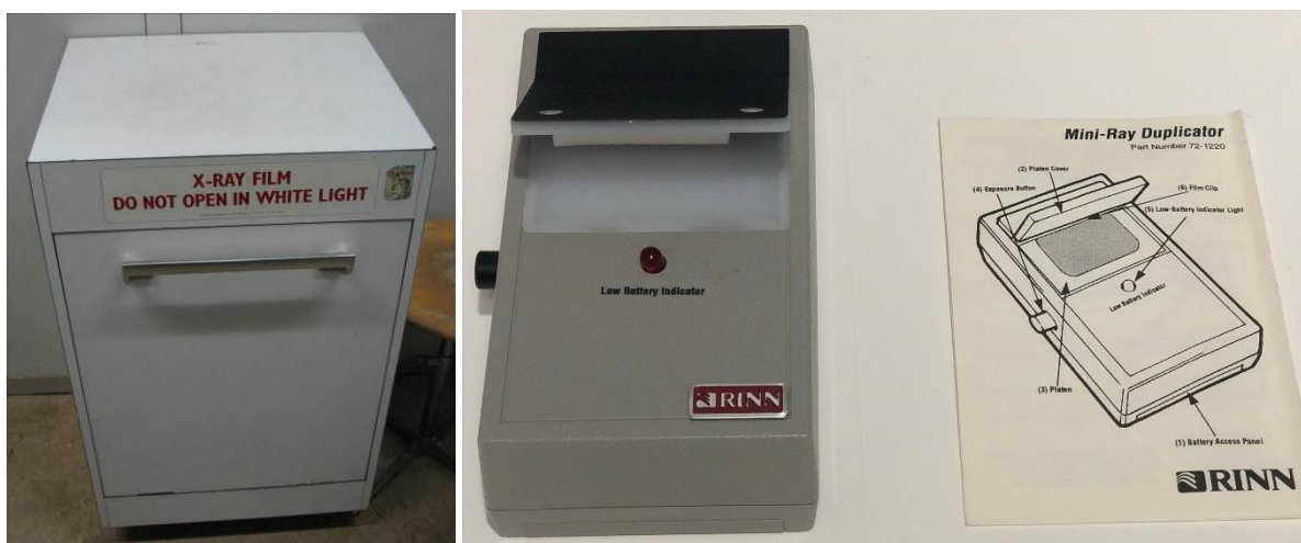
Fig. 72 Left: Radiograph copying machine. Courtesy of A. Al-Ekrish (King Saud University) Right: intra-oral film duplicator. Courtesy of S. Anamali (University of Iowa).
