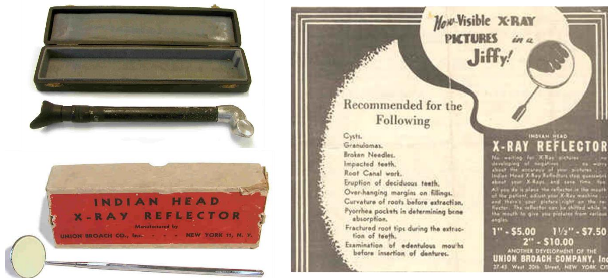
Fig. 14 Top left: the Dentoscope, an intra-oral fluoroscope produced in Switzerland (ca. 1930s). Bottom left: the Indian Head X-ray Reflector of the Union Broach Company (US, ca. 1955). Distribution was halted by the State of New York. Pictures and information provided by the Oak Ridge Associated Universities (ORAU) Health Physics Historical Instrumentation Museum Collection under a non-transferable, non-exclusive, limited license [44,45].
