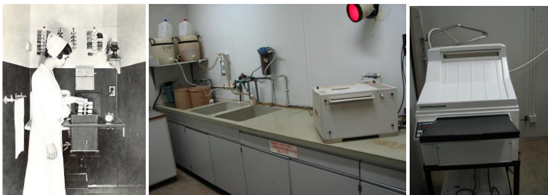
Fig. 36 Left: A dental assistant (hygienist) developing an X-ray film (original source and year unknown). Middle and right: automatic processors for intra-oral films and large films. Courtesy of A. Al-Ekrish (King Saud University).
