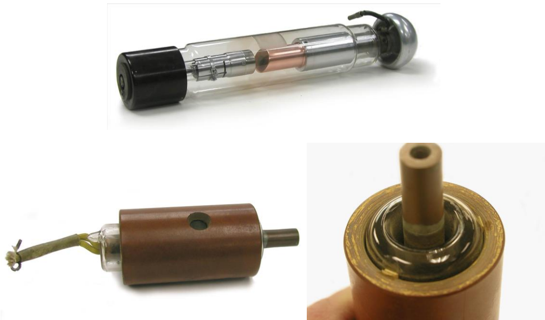
Fig. 22 Top. Single focus dental XPD Coolidge tube (General Electric, ca. 1930s-1940s). Bottom: shock-proof dental x-ray tube (likely by General Electric, ca. 1935) [57]. The housing is made of several lead layers, separated by an insulating material. Figures and information provided by the Oak Ridge Associated Universities (ORAU) Health Physics Historical Instrumentation Museum Collection under a non-transferable, non-exclusive, limited license [58,59].
