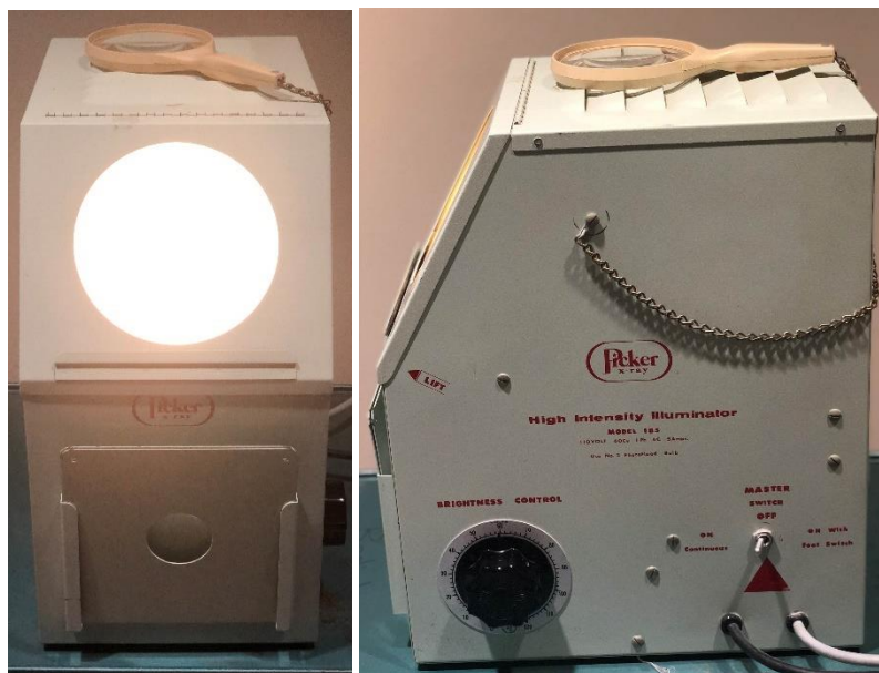
Fig. 70 High intensity illuminator (Picker X-Ray, USA) with attached magnifying glass. Courtesy of S. Anamali (University of Iowa)
