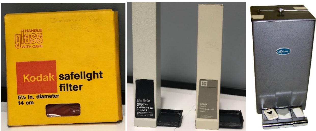
Fig. 38 Left: Safelight filter for intra-oral films. Middle: Kodak dental film dispenser. Courtesy of S. Anamali (University of Iowa). Right: Rinn dental film dispenser. Courtesy of D. Bednarek (University at Buffalo).
