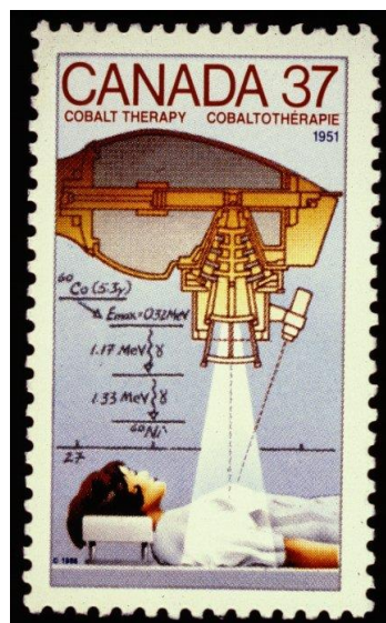
Figure 14. Canadian postage stamp recognizing the development of cobalt-60 radiation therapy in Canada and the involvement of Harold Johns in that development. The stamp includes a schematic of a typical head of a cobalt-60 machine. The source shutter mechanism is a sliding drawer. The source is shown in the “on” position. To turn the beam “off”, the source drawer is slid to the left. Also shown is the decay scheme of cobalt-60 with a beta decay with a maximum energy of 0.32 MeV followed by 2 gamma rays of 1.17 and 1.33 MeV. This style of machine was the most produced and used globally. Canada Post © 1988. Reproduced with permission.
