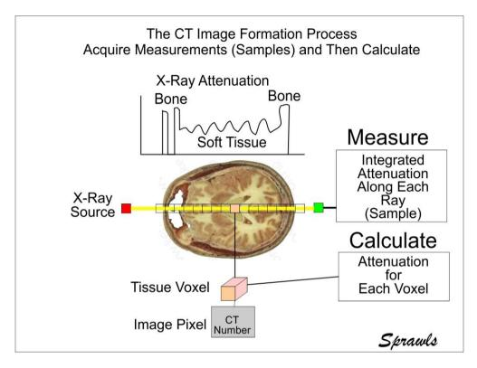
Fig. 6. The two phases in the formation of CT images, measuring and acquiring data followed by calculating attenuation values for each voxel. The illustration is for one ray through the body but many (100s) are required to produce an image.
