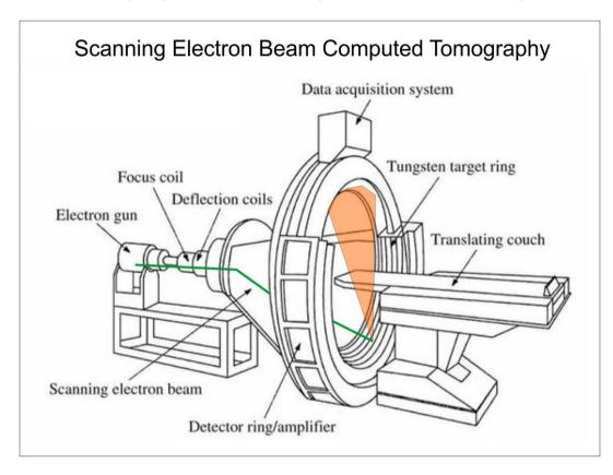
Figure 22. The scanning electron beam design that provides rapid scanning.
