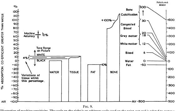
Illustration of machine sensitivity. The scale on the right is an arbitrary scale used on the print-out and is related to water = 0, air = 500 units. It can be seen that most materials to be detected fall within 20 units above zero and can be covered by the adjustable 4 per cent "window".
