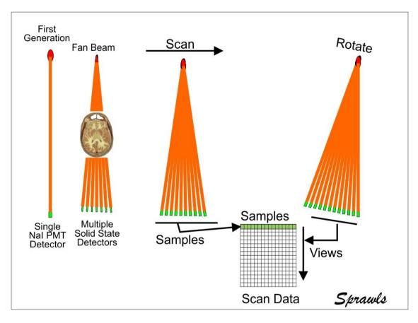
Figure 19. The geometry of the second-generation technology using an array of multiple detectors.
