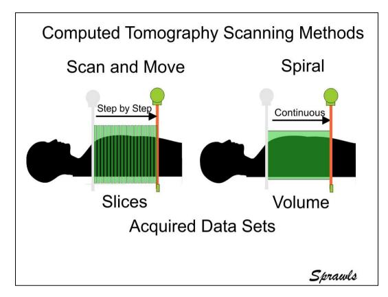
Fig. 26. Comparing scanning methods and acquired data sets.
