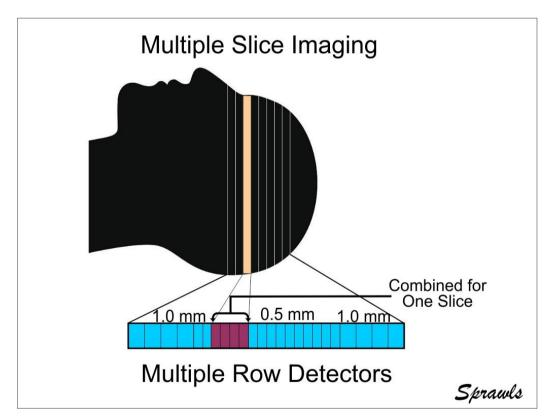
Fig. 24. Multiple Row Detectors and Multiple Slice Imaging
