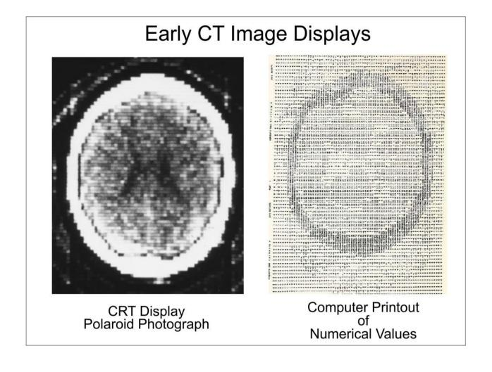
Fig.13. The two types of image displays for the first CT scanners.
