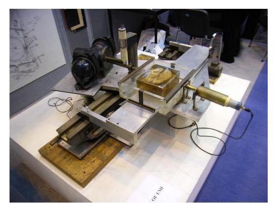
Fig. 11. Hounsfield's laboratory device used in the development of the computed tomography method.
