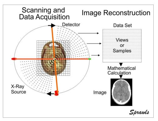
Fig.5. The two phases of CT, scanning and acquiring data that is then used to mathematically calculate, or reconstruct, an image.
