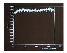
Fig. 4 Profile indicates problem of scanning mechanism.
