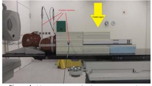
Figure 1. Measurement setup for the prostate cases using an anthropomorphic phantom and stacks of solid water equipped with ionization chambers for peripheral dose measurements and a 2D array for plan verification. The yellow arrow indicates the treated region [2].
