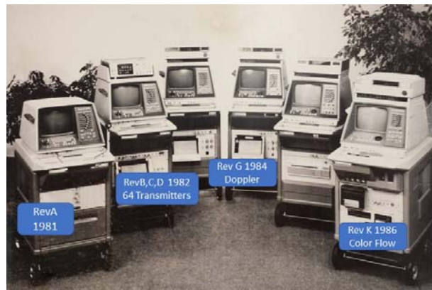
Fig. 11 HP imaging system upgrade path from 1981 to 1986 (Illustration by courtesy of Koninklijke Philips N.V and annotated by Karl Thiele).
