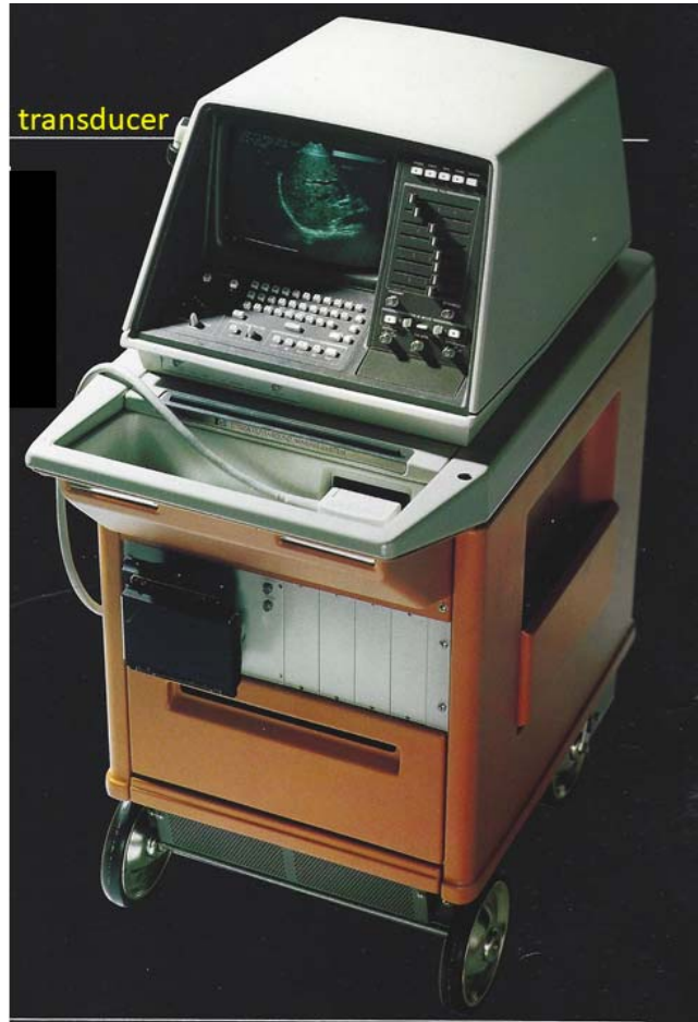
Fig. 5 Hewlett Packard 77020A phased array ultrasound cardiac imaging system with transducer shown on left side ( Illustration by courtesy of Koninklijke Philips N.V).
