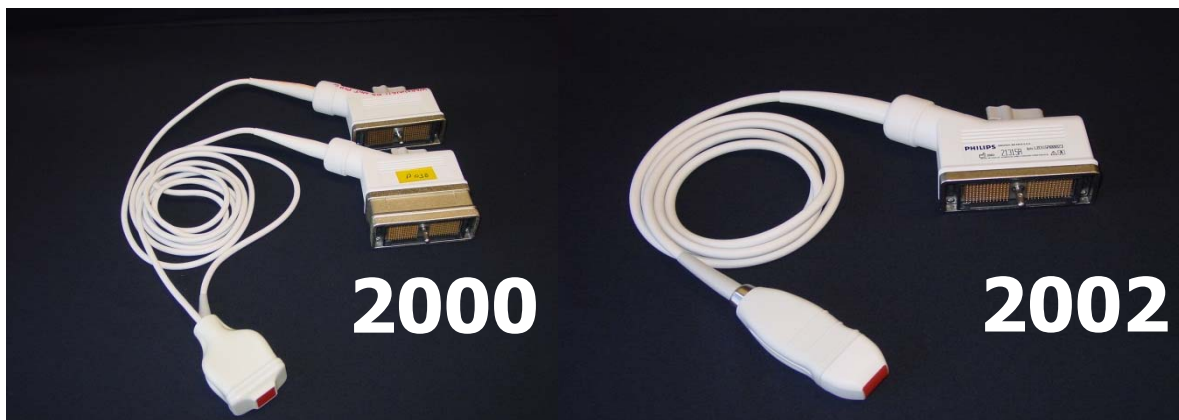
Fig. 13 Matrix arrays with microbeamformers in the handle: A.(left) first working prototype B. (right) close to final product (Courtesy of Karl Thiele).
