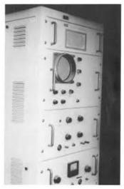
Fig. 4. First commercial Doppler ultrasound system; the 'Blood Rheograph' available in 1959 and developed by the Nippon Electric Company (Japan). Reproduced from Ultrasound Med Biol, Vol. no. 12, Kaneko Z, First steps in the development of the Doppler flowmeter, pp. 187-195, copyright Elsevier (1986).
