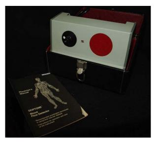
Fig. 6. Doptone CW Doppler system manufactured by the Smith-Kline Instrument Company (Philadelphia, USA). The system was the first fetal heart monitor. The version illustrated was used in peripheral vascular applications. Reproduced with permission from the British Medical Ultrasound Society.
