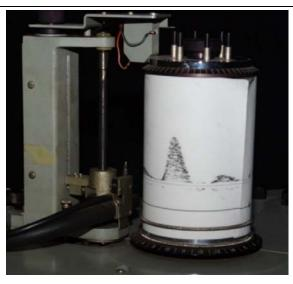
Fig. 7. Spectral Doppler tracing made by the Kay Spectrograph (Kay Electric Company, Pine Brook, USA). The tracing is in-place on the paper attached to the recording drum of the machine. Reproduced with permission from the British Medical Ultrasound Society.
