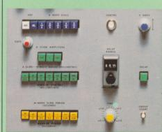
Pushbutton automatic centering of image, colour coded controls of 'B' Scan, 'A' Scan and 'M' mode operations.
