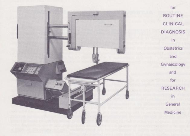
The Diasonograph is a multi-purpose system for the investigation of soft-tissue structures in the body by pulsed ultrasonic waves. The operating principle is basically the same as that of underwater echo sounding or 'sonar'. However, the sound waves used have a much higher frequency, corresponding to a wavelength in tissues of 1 mm or less.
