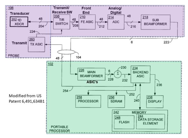
Fig. 14 Block diagram for portable ultrasound imaging system with sub-beamformers in probe handle (From US Patent 6,491,634B1).
