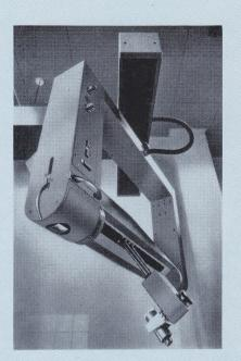
Positioning of the scanning plane is achieved with push-button controlled magnetic locks (Courtesy Design Magazine and Philip Sayer)
