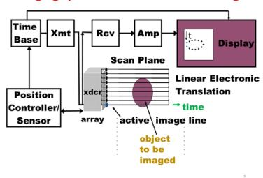
Fig. 1 Basic setup for B (Brightness)-mode imaging in which elements in an array are sequentially switched to produce image lines. (From [8])
