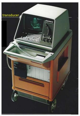
Fig. 5 Hewlett Packard 77020A phased array ultrasound cardiac imaging system with transducer shown on left side (Illustration by courtesy of Koninklijke Philips N.V).
