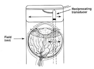
$Fig.\ 10\ A\ schematic\ diagram\ of\ an\ oscillating\ transducer,\ real-time\ B-scanner.\ The\ oscillations\ produce\ a\ linear\ scan.$
