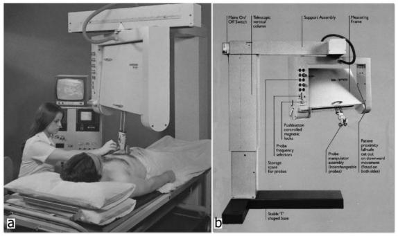
Fig. 26 a) The EMISONIC 4200 Diasonograph. b) Annotated image of the mechanical system. From Nuclear Enterprises Bulletin No. 112 (1977) [70].
