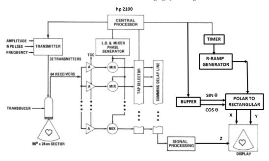
Fig. 4 HP Labs prototype ultrasound imaging system block diagram circa January, 1977([16 17] and modified courtesy of Ed Karrer).
