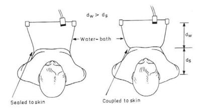
Fig. 4 Water-bath coupling techniques.
