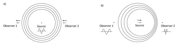
Fig. 1. Doppler effect; there is relative movement between the source and the 2 observers. a) Wave motion with respect to the source. The wave propagates symmetrically in all directions at a frequency f. b) Wave motion with respect to the observers. Wave propagation is asymmetric; there is contraction of the wave as perceived by Observer 2 who perceives a higher frequency  $(f_1 > f)$ ; for Observer 1 there is dilation of the wave who perceives a lower frequency  $(f_1 < f)$ .
