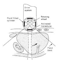
Fig. 8 A schematic diagram of a rotating transducer, real-time B-scanner.
