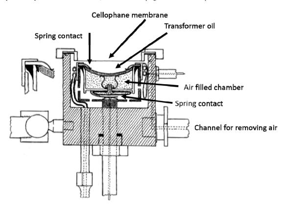
Fig. 3 Transducer mount used by Lynn et al (11).
