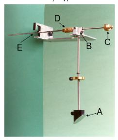
Fig. 6 Equilibrium balance for measuring radiation force
