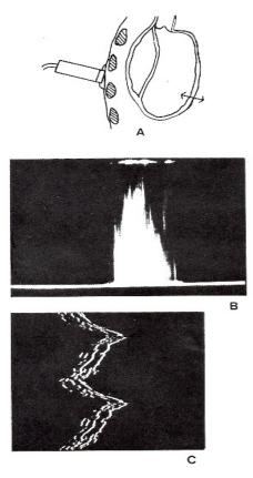
Fig. 2 Principle of M-scanning. (a) Transducer directed at moving structure of interest and held fixed, (b) echoes may be observed on an Ascan display but this does not give a record of motion, (c) echo dots sweep up the screen to provide a trace of position versus time.
