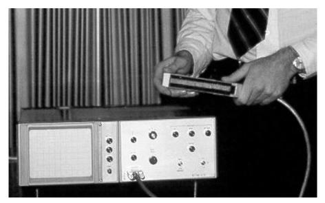
Fig. 35. The popular 61-channel ADR linear array scanner, produced by the Advanced Diagnostic Research Corporation in the USA, in 1973. Photo courtesy of the BMUS Historical Collection.
