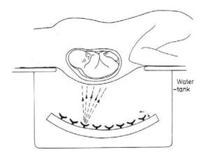
Fig. 5 Basic structure of the UI Octoson scanner.
