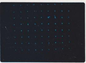
Cross-sectional picture of a matrix of wires spaced at 0.5in (12.7mm) intervals in a water tank
