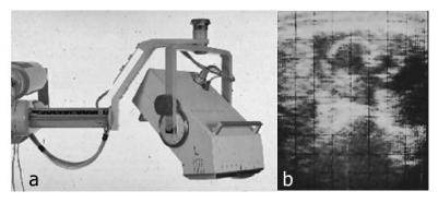
Fig. 33. a) The 'Vidoson' real-time water-bath scanner, was commercially introduced by Siemens Medical Systems, Germany, in 1965. As each of three transduces was rotated around the focal line of a parabolic mirror, its reflected beam was swept across the aperture, remaining parallel to the principal axis. b) An example of a single frame from an obstetric patient. Courtesy of the BMUS Historical Collection.
