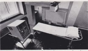
In the new Diasonograph, maximum use has been made of floor space without any sacrifice in the facility of selecting the more difficult scanning planes. The construction of the scanning system and the control cabinet affords considerable freedom of choice in the layout of the examination room. Total system weight is 650kg. (Photo courtesy Design Magazine and Philip Sayer)
