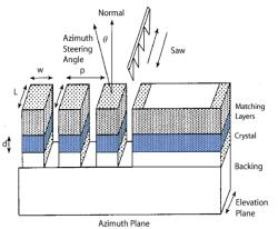
Fig. 8 Array construction showing elements of period p and width
