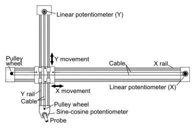
Fig. 14 Illustrating the principle of the system used to support and constrain the probe within the scan plane and to obtain the X,Y and angle coordinates of the probe relative to the scan plane.
