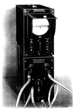
Fig. 1 The Kelvin and Hughes Mark IIb Flaw Detector.
