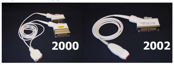
Fig. 13 Matrix arrays with microbeamformers in the handle: A.(left) first working prototype B. (right) close to final product (Courtesy of Karl Thiele).
