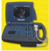
Fig. 15 OptiGo portable low cost ultrasound imaging system released by Philips in 2002 (Illustration by courtesy of Koninklijke Philips N.V).
