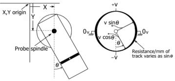
Fig. 9 Left: Measurement of probe angle  $\Theta$  relative to the Y axis of the scan plane. Right: The 'cosine' wiper of the sine-cosine potentiometer is at the same angle as the principal axis of the probe.
