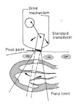
Fig. 9 A schematic diagram of an oscillating transducer, real-time B-scanner. The oscillations produce a sector scan.
