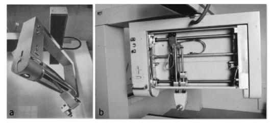
Fig. 23. a) Patient's view of the probe, the probe support box and the outer frame of the box, on an NE 4102. From Nuclear Enterprises Bulletin No. 64 [60]. b) View of the interior of the probe support box. The X and Y guide rails shown schematically in Figure 14 are prominent. Photo courtesy of the Design Council Slide Collection at Manchester Metropolitan University Special Collections.
