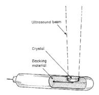
Fig. 12 Transducer for 360° radial invasive scanning.
