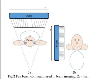
Fig.2 Fan beam collimator used in brain imaging. 2a - Beam Collimator in the radial direction 2b - Fan Beam Collimator in the z direction
