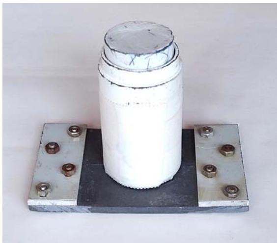
Fig. 1 Slit phantom with encapsulated source.
