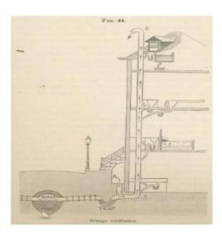
The significance of properly designed and constructed sewer systems is emphasized here in Fig. 44. A specific Health issue illustrated here is proper venting to protect against the buildup of gases in the living areas.
