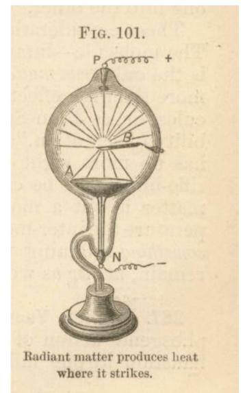
The tube shown in Fig. 101 was used to demonstrate that radiant matter produced heat when it was absorbed in a material. It contained a small platinum plate at the positive terminal (B) and a focused cup at the negative terminal as shown. When it is connected to an electrical source radiant matter is focused on the platinum plate heating which becomes red-hot. The heat radiates to the glass tube causing it to become warm.
