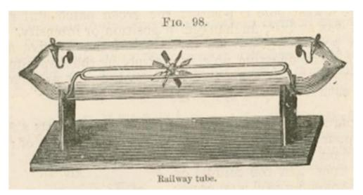
The apparatus shown in Fig. 98 was used by Professor Crookes to demonstrate that radiant matter could exert forces and names this the Railway Tube. It consists of a track running between the two electrodes at the ends of the tube.
