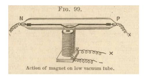
The tube shown in Fig. 99 was used to demonstrate that radiant matter could be deflected with a magnet. Within the tube there was a partial vacuum leaving sufficient gas to ionize and glow along the path of radiant matter between the two electrodes.
