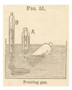
It is generally easy to pour a liquid from one container to another with the help of gravity. How do you pour a gas? One method used in the physics laboratory is illustrated here. It is done in a large container of water. An empty container, with respect to gas, is filled with water and with the opening down in the larger water container. When a gas is poured from another container it displaces the water as it bubbles up into the receiving container.
