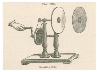
Newton's rotating disk shown in Fig. 226 is one method used to demonstrate the composition of light as a mixture of different colors. Disks divided into segments of various colors are mounted on the spinning apparatus. When they are spun at a high speed the composite color is observed. This would be white when the segments of the disk contain the spectrum of colors that are in white light.
