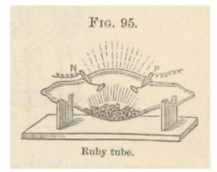
Shown here in Fig. 95 is the Ruby Tube developed by Professor Crookes. Various substances are placed in the highly evacuated (about one millionth of an atmosphere). When the electrodes are connected to a coil providing a high voltage the
