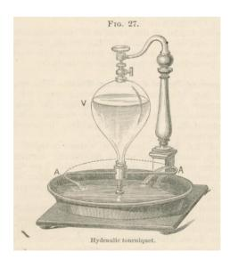
One of the principles of hydrodynamics, or fluid in motion, is demonstrated in Fig. 27. Specifically, that forces are created by moving fluid. The hydrostatic pressure in the glass container forces water out through the small openings at the end of the tubes.
