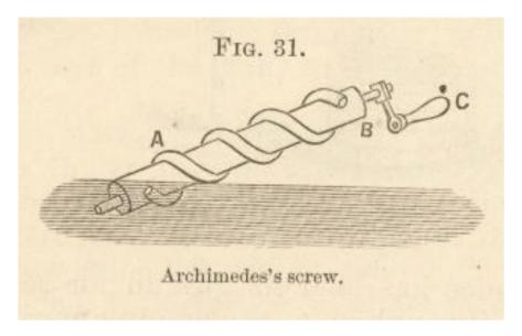
Hydraulics, the movement of fluids, is achieved with many different devices, including pumps, turbines, etc. One method uses an Archimedes's screw illustrated in Fig. 31. It was used extensively, especially in Europe, to pump water, drain flooded areas, and to move sewage.
