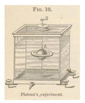
The experiment shown in Fig. 10 uses a quantity of olive oil suspended in a mixture of water and alcohol that had the same density as the oil. This eliminated any influence of gravity. The oil assumes a spherical shape as show. When it is spun by hand with the handle a satellite ring is formed. This is similar in form to the satellite ring around Saturn.
