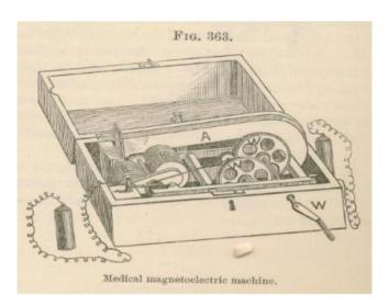
The principle of magnetic induced currents was used to explain the operation of the "magnetoelectric" machine shown in Fig. 363. It contains a large horse-shoe magnet (A) and a mechanism for rotating a small metal object between the magnetic poles. As the magnetism in the object fluctuates with the rotation, an electric current is induced in a coil around the rotating object. The machine was used to pass electrical currents through the human body for medical purposes.
