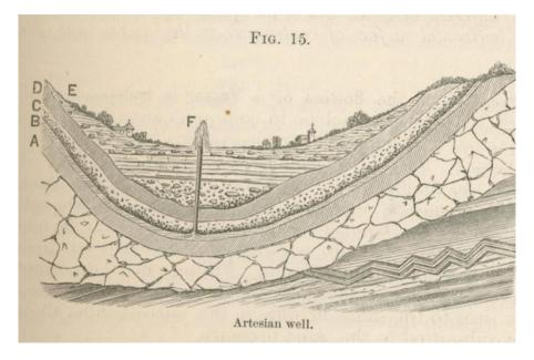
The sources of water for so-called Artesian wells are often distances away and always at higher elevations as illustrated in Fig. 15. The community health issue is the water is coming and filtered through channels and generally not contaminated as water from shallow wells might be.
