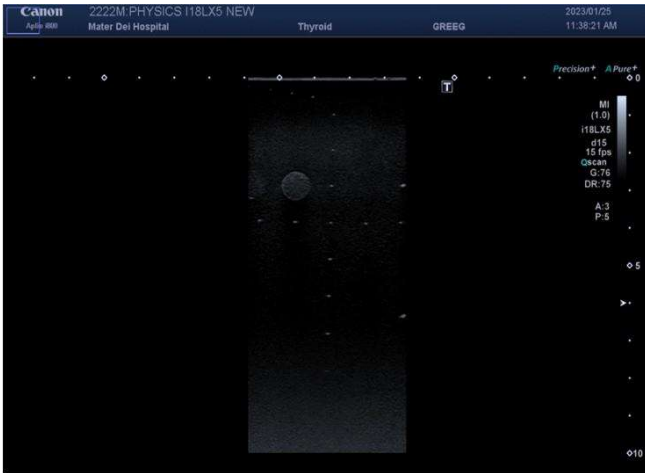
Fig. 2: An ultrasound image using a linear transducer on the Canon Aplio i8000
