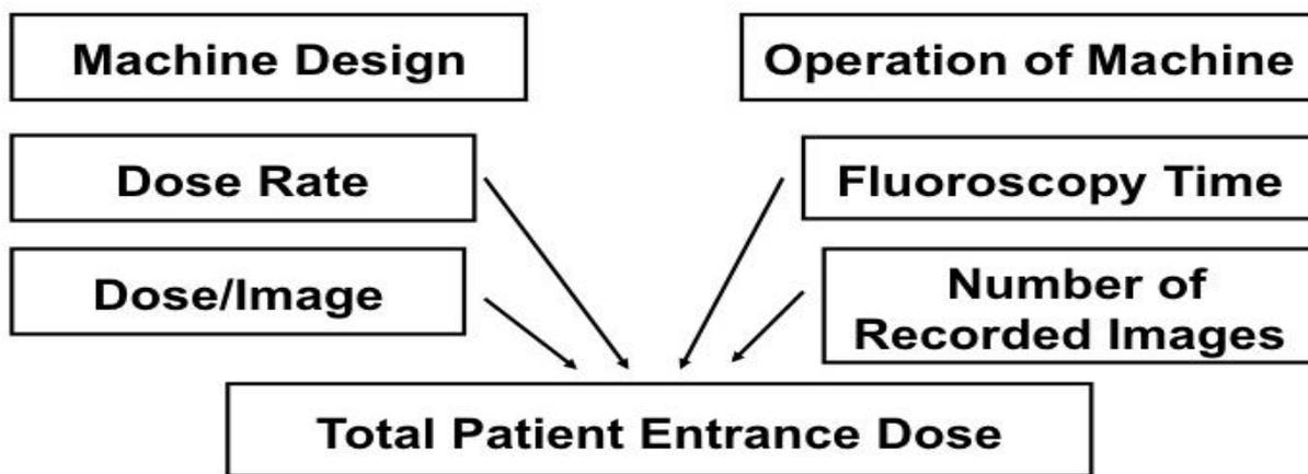
Fig. 8: Total patient entrance dose from a fluoroscope depends on the dose rate during fluoroscopy and dose per recorded image, both factors dependent on the fluoroscope's design and configuration. Total patient entrance dose is also directly related to fluoroscopy time (number of fluoroscopic images) and number of recorded images, which are more dependent on the training and experience of the operator than on the fluoroscope's design and configuration.
