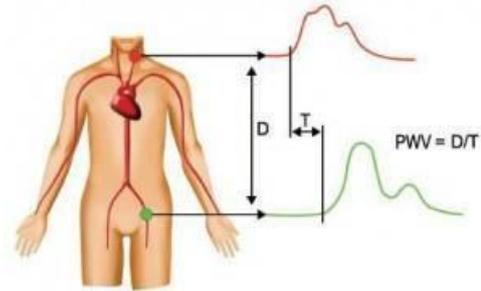
Fig. 13 Classical tonometry measurement methodology (from ref [31])
