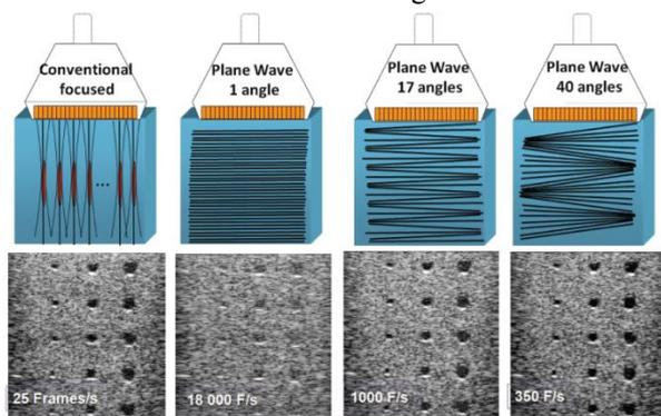
Fig. 3 From conventional line per line imaging to ultrafast coherent compound (from ref [3])
