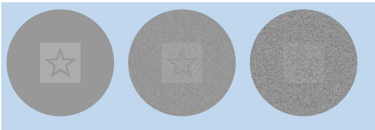
Fig. 12: The image on the left is produced with a radiation dose to the patient more than an order of magnitude greater than the image on the right. The central image is the correct configuration: diagnostic image quality at a properly managed radiation dose
