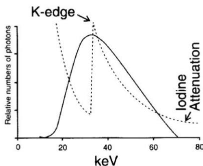
Fig. 11. Iodine Attenuation compared to the effective energy of a 70 kV X-ray Beam Spectrum with 3 mm aluminum total filtration. The effective energy of the x-ray beam spectrum, ~ 30 keV, is well matched to the 33 keV k-edge of iodine. This matching increases the radiopacity of an iodine-filled vessel. Reprinted with permission. [83]
