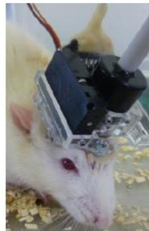
Fig. 16 Portable functional brain imaging system (from ref [37])
