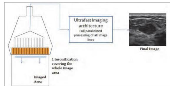
Fig. 2 Basic Principle of Ultrafast Imaging scanners (from ref [2])
