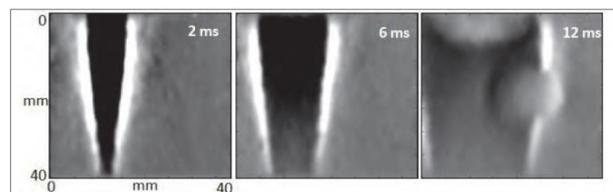
Fig. 4 Plane shear wave along a Mach cone from a supersonic source propagating in a heterogenous phantom (from ref [2])
