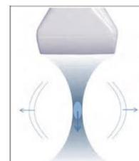
Fig. 1 Acoustic radiation from an ultrasound beam (from ref [3])
