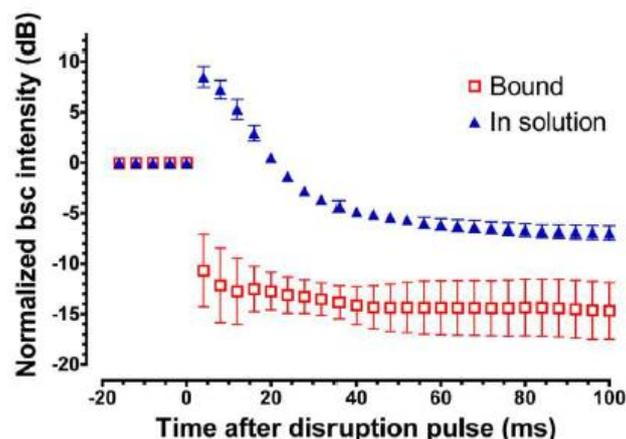
Fig. 17 Dissolution time of bounded and free bubbles in a phantom after a disruption pulse (from ref [38])
