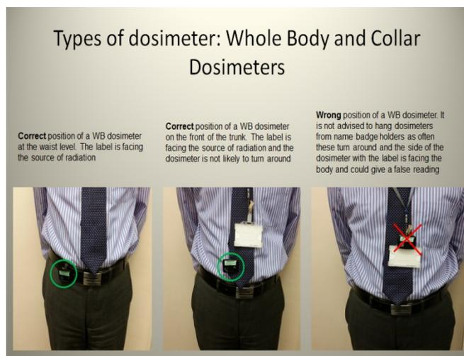
Fig. 1 Correct and wrong positioning of a whole body dosimeter
