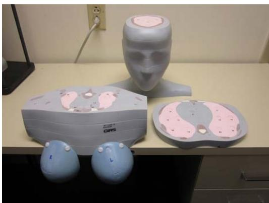
Fig. 6 An example of an anthropomorphic phantom (ATOM model 702; CIRS, Norfolk, VA, USA); it has holes for inserting small dosimeters
