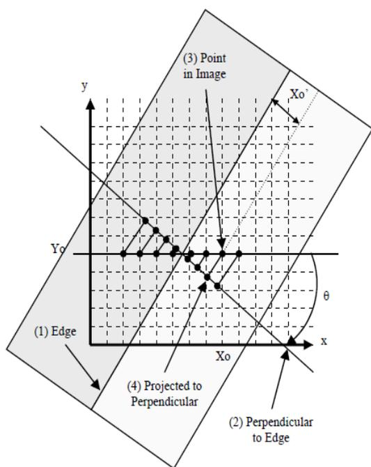
Figure 1: ESF registration onto a reference point
