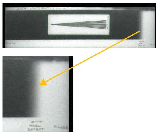
Fig.5 Illustration of Heel effect in old X-ray tube (gradual drop of optical density at the right side of radiograph). Note the zoom of the Heel effect zone (below), which is usually about 2-5 mm wide on the radiograph recording the effect.
