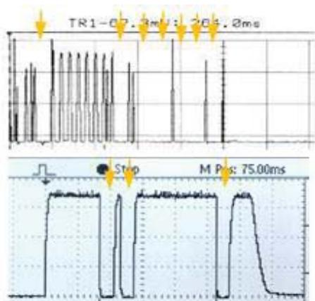
Fig.3 kVp oscillograms of X-ray tubes during arcing (see arrows)
