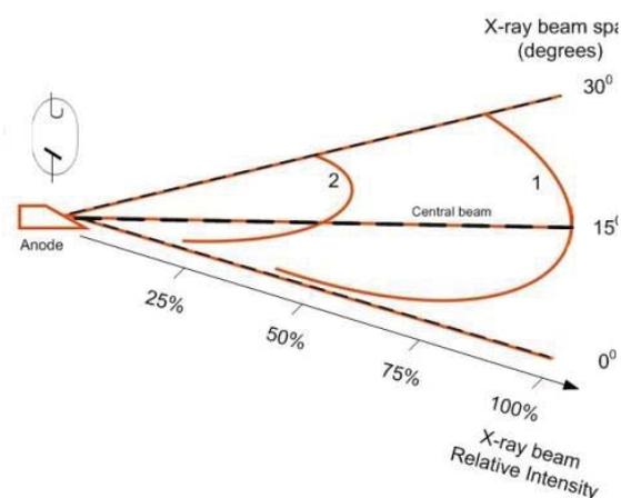
Fig.4 X-ray tube intensity spatial distribution for new X-ray tube (curve 1) and an old one (curve 2). The X-ray intensity is shown in relation to the maximum intensity (100%) at the middle of the central beam of a new X-ray tube. Note also the shifting of the maximum of the intensity from the central beam ( $15^{\circ}$ ), what leads to significant decrease of the beam intensity at the side of the Anode – i.e. increased Heel effect.
