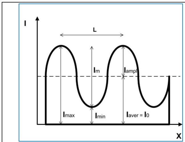
Fig.2 Intensity (I) of the X-rays after their modulation by a hypothetical phantom with the above sinusoidal shape. X is related to the dimensions of the phantom. L is the period of the phantom structures.
