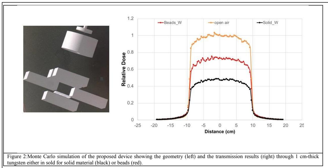
Figure 2: Monte Carlo simulation of the proposed device showing the geometry (left) and the transmission results (right) through 1 cm-thick tungsten either in solid for solid material (black) or beads (red).
