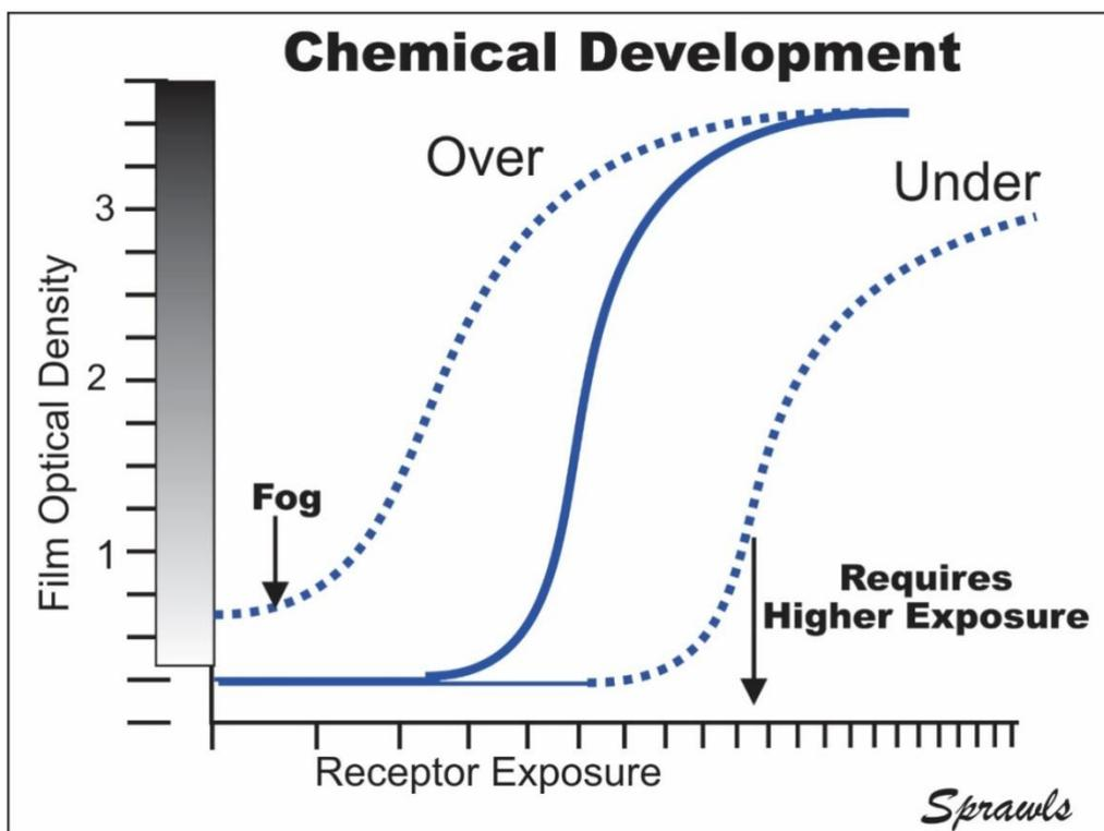
Figure 11. The effects of incorrect levels of development on film characteristics.
