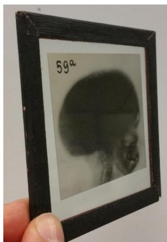
Figure 4.a Radiographs recorded on a glass plates being chemically processed. They are rigid, fragile, and relatively heavy to handle
