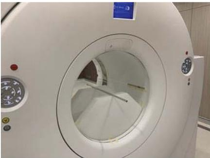
Figure 5 Sensitivity phantom 5 layers of metallic cylinder inserted by polyethylene tube of  $700 \pm 20$  mm filled with  $^{18}\text{F}$  solution. Acquisitions of 5,4,3,2 and 1 layers at center and 10 offset of FOV
