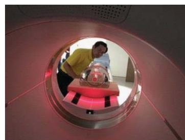
Figure 8 Setup for IEC/2001 body phantom and line source in scattered phantom for image quality acquisition
