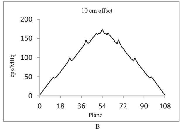
Figure 6 A) Axial sensitivity profile at center of FOV B) at 10 cm off center
