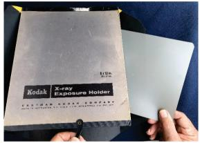
Figure 13. Industrial type film being inserted into a cardboard holder to be used as a receptor for mammography.
