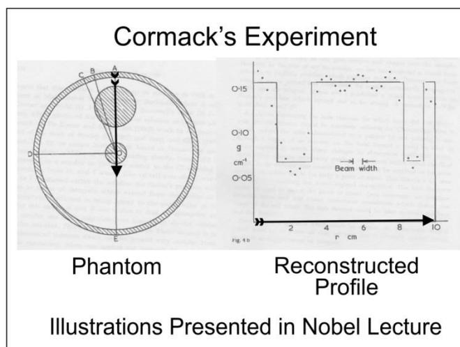
Fig. 9. Diagram of phantom scanned and reconstructed profile of attenuation along a pathway through the phantom as illustrated. The dots representing the calculated values are compared to the actual values represented by the solid line.
