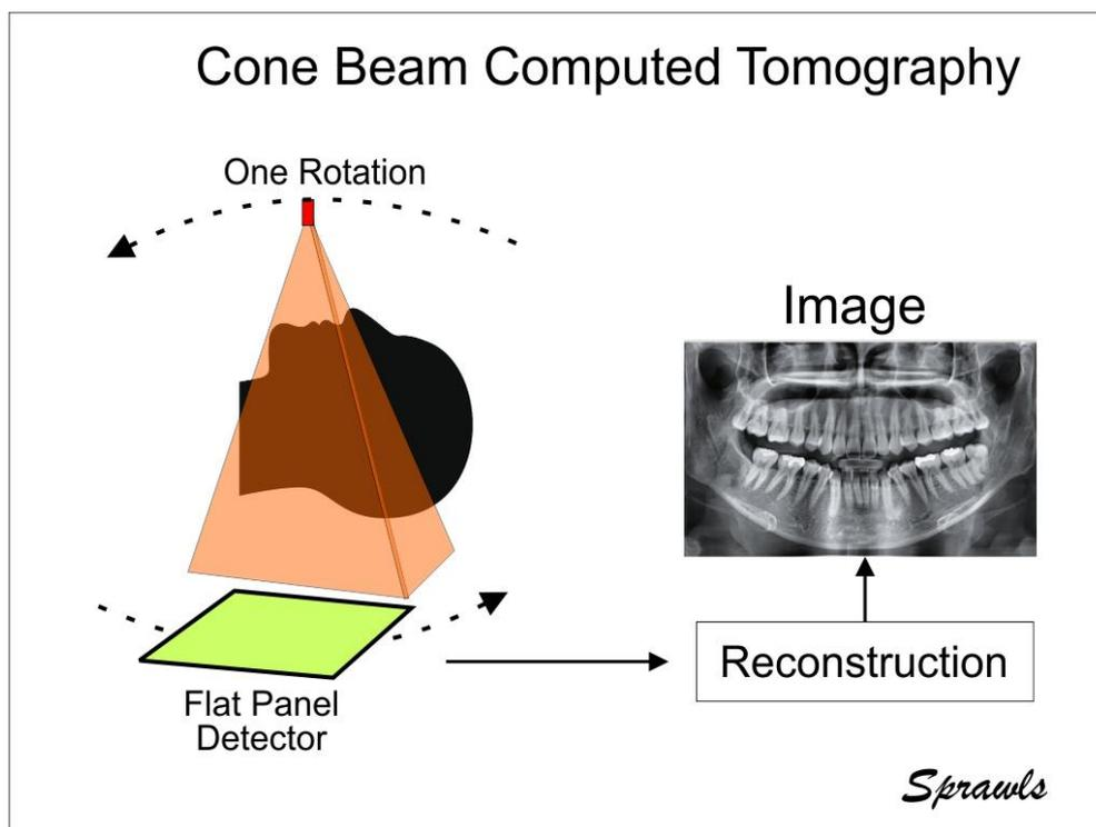
Fig. 29. The concept of cone beam computed tomography.
