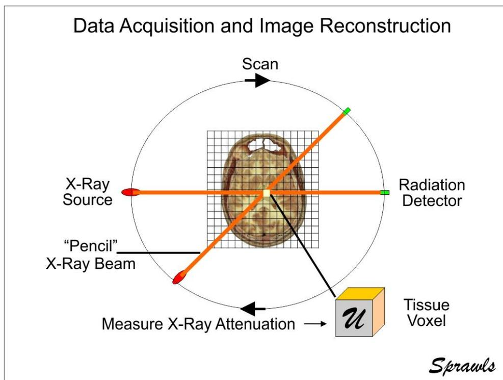
Figure 17. The objective of data acquisition by scanning and mathematical reconstruction is to determine the x-ray attenuation values for each individual tissue voxel within the imaged slice.
