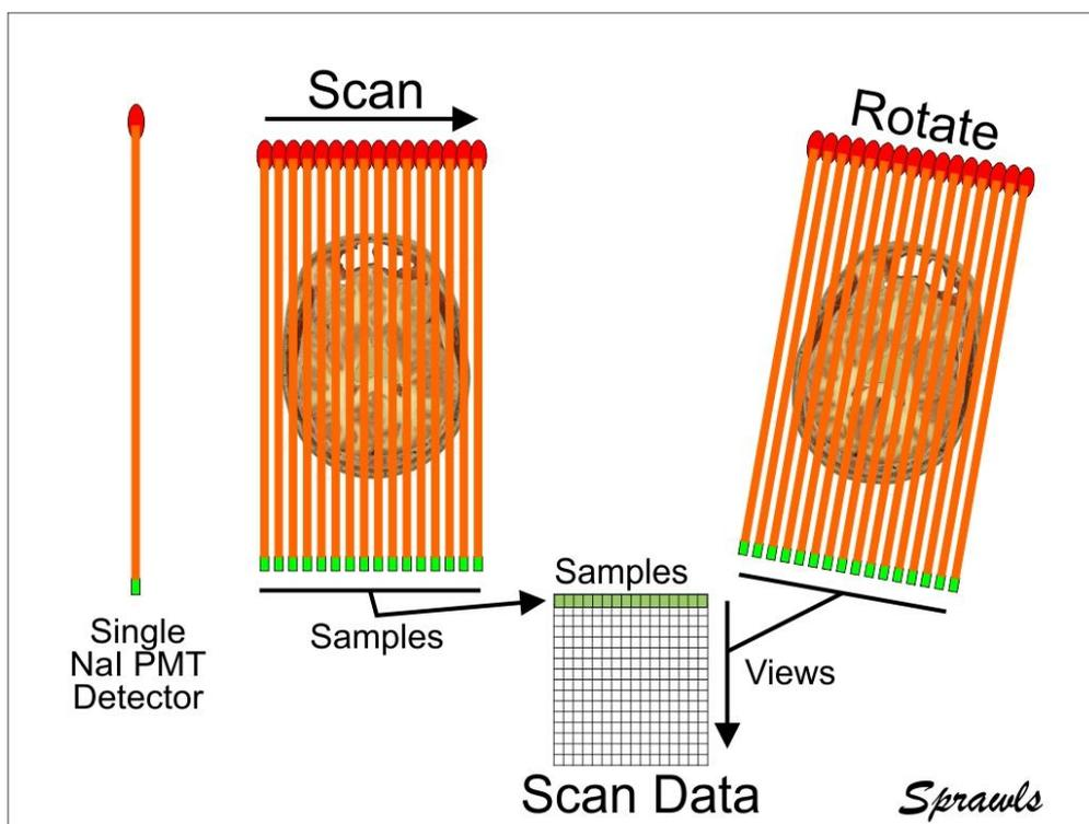
Figure 18. The scanning geometry for the first-generation CT scanner.
