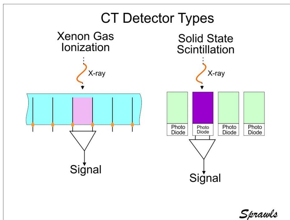
Figure 23. A comparison of the two detector types.
