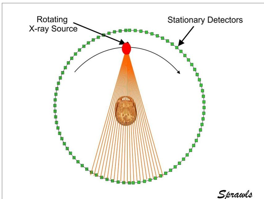
Figure 21. A large circular array of detectors that does not need to be moved.
