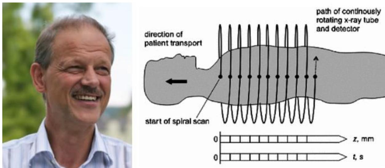
Fig. 25. Dr. Willi Kalender and diagram illustrating the spiral scanning process.
