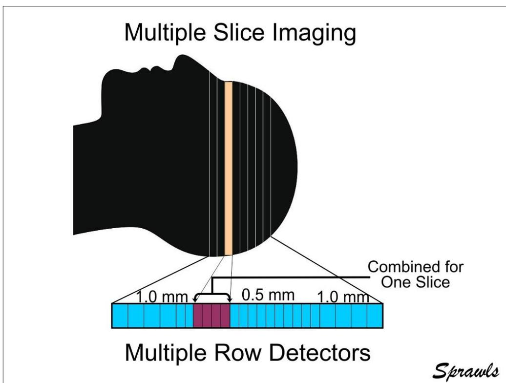
Fig. 24. Multiple Row Detectors and Multiple Slice Imaging
