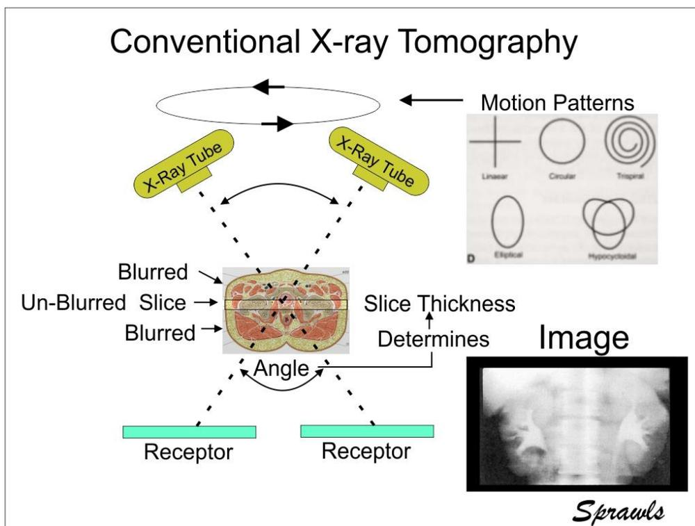
Fig.3. An overview of the conventional x-ray tomography process.
