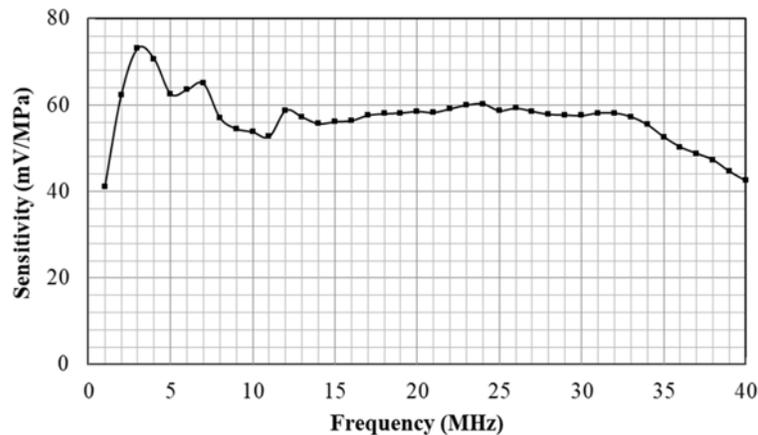
Fig. 13 Amplitude response of a 9  $\mu\text{m}$ , 0.2 mm diameter PVDF needle hydrophone. (Courtesy of Dr A Hurrell, Precisions Acoustics, Dorchester, UK)
