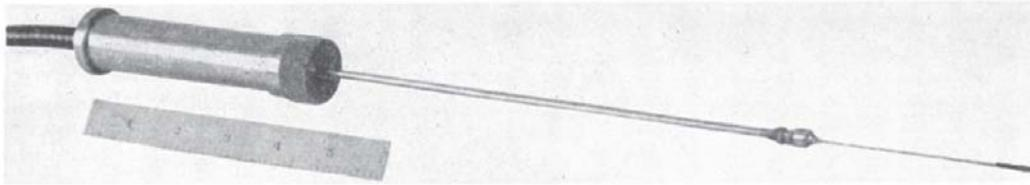
Fig. 4 The probe hydrophone of Mellen (1956) [11]. (Reprinted with permission from Mellen RH. An experimental study of the collapse of a spherical cavity in water. *J Acoust Soc Am* 1956; 28: 447. Copyright 1956, Acoustic Society of America.)
