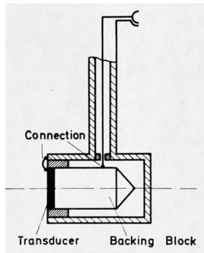
Fig. 5 A general hydrophone design for pulsed diagnostic beams. (From Brendel 1972). [15]
