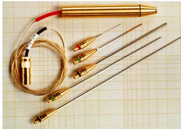
Fig. 9 A set of early Precision Acoustics needle hydrophones. The hydrophones could be connected interchangeably into the submersible preamplifier shown at the top of the picture. (Image courtesy of Dr A Hurrell, Precisions Acoustics, Dorchester, UK)
