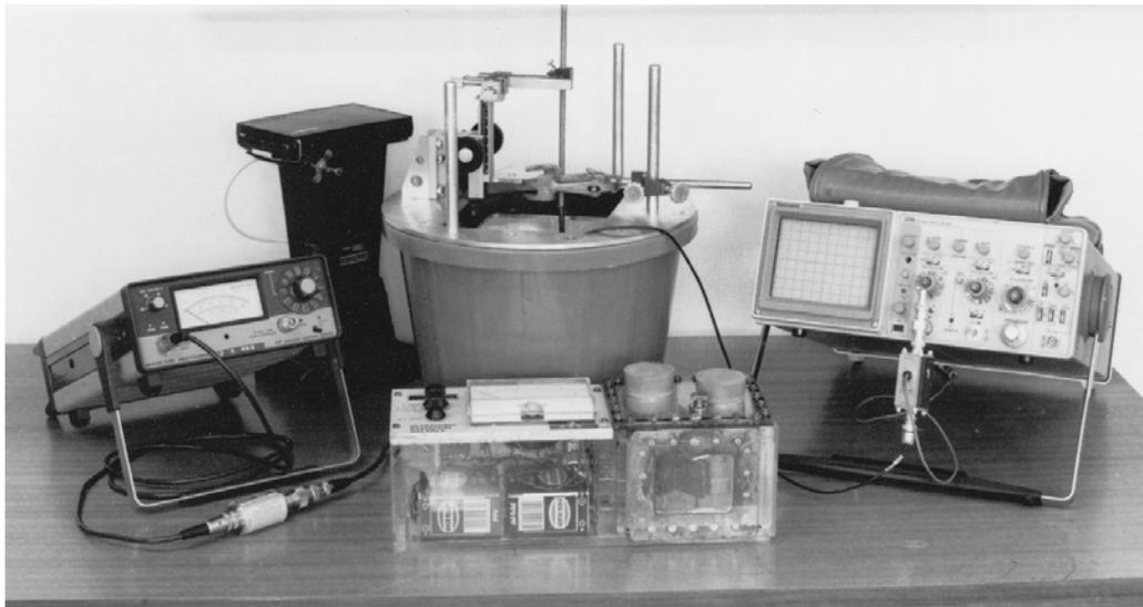
Fig. 16 Portable measurement system used to make acoustic output measurements on clinical ultrasound machines in the Northern Region, including the RF power meter (left) and Farmery and Whittingham radiation force balance (centre front). The membrane hydrophone is mounted inside the water bath (centre rear).
