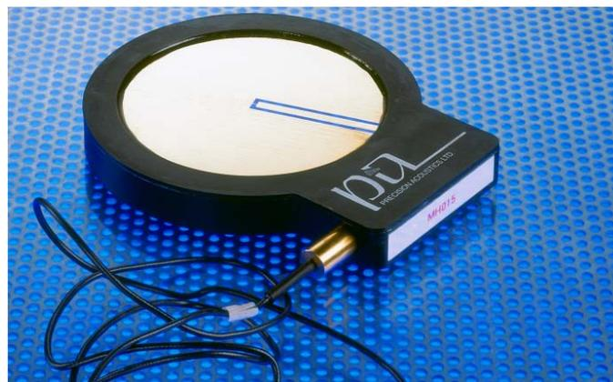
Fig. 10 An early model of Precision Acoustics bilaminar membrane hydrophone. (Image courtesy of Dr A Hurrell, Precisions Acoustics, Dorchester, UK)
