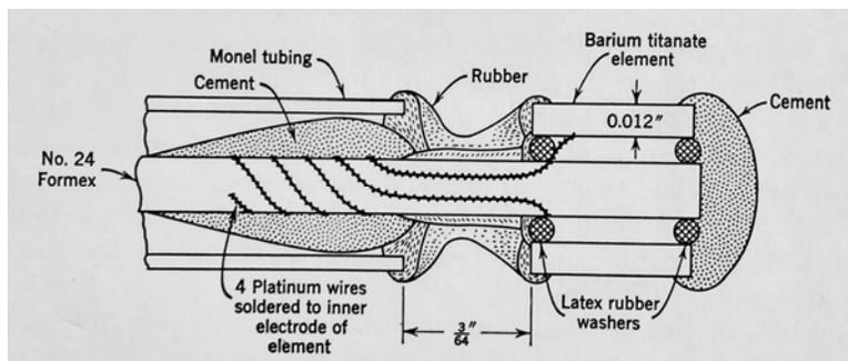
Fig. 3 A miniature piezoelectric ceramic hydrophone based on a small barium titanate cylinder element. (From Hueter and Bolt 1955)[10]
