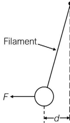
Fig. 12 The elastic sphere radiometer suspended in a sound field.
