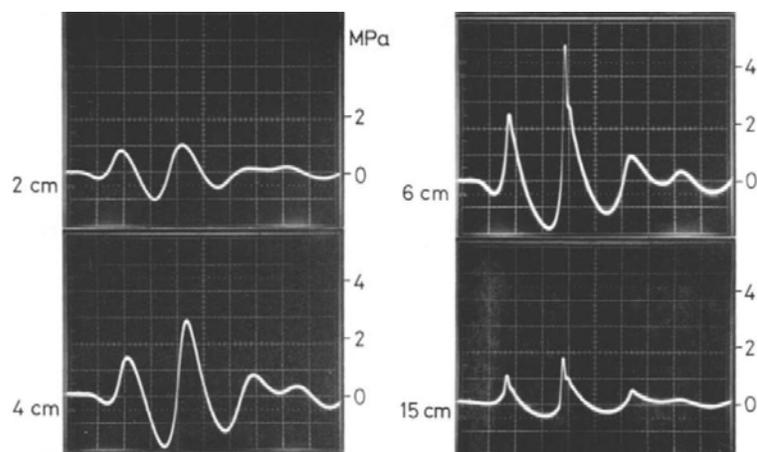
Fig. 11 The pressure pulse measured in the field from a focused 2 MHz transducer at 2 cm, 4 cm, 6 cm and 15 cm range. (From Duck FA, Starritt HC. Acoustic shock generation by ultrasonic imaging equipment. *Brit J Radiol* 1984; 57: 231-40.) [35]
