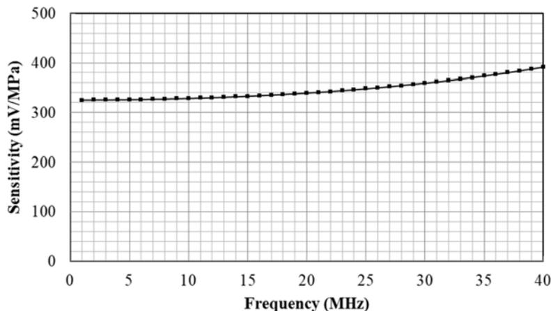
Fig. 14 Amplitude response of a 16  $\mu\text{m}$ , 0.4 mm PVDF differential membrane hydrophone. (Courtesy of Dr A Hurrell, Precisions Acoustics, Dorchester, UK)
