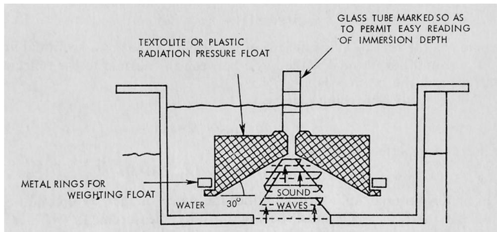
Fig 12. Henry's design for a power balance using a neutral buoyancy absorbing float target. 1957. [24] (©Iiffle Books Ltd)
