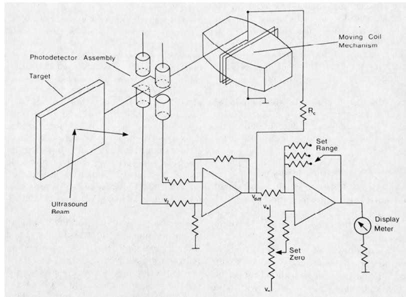
Fig 16. The servo-controlled circuit of Farmery and Whittingham. 1976 [45]. Permission to reproduce: Elsevier Inc.
