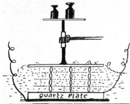
Fig 4. Sketch diagram showing the principle of weighing the variation of radiation force in a standing wave. Wood, 1939. [11]
