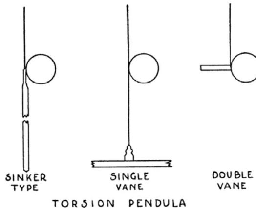
Fig 2. Various designs of torsion pendulum targets. [4]
