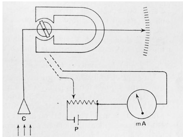
Fig 15. Dognon's electromagnetic feedback technique to measure radiation force. 1953. [39].
