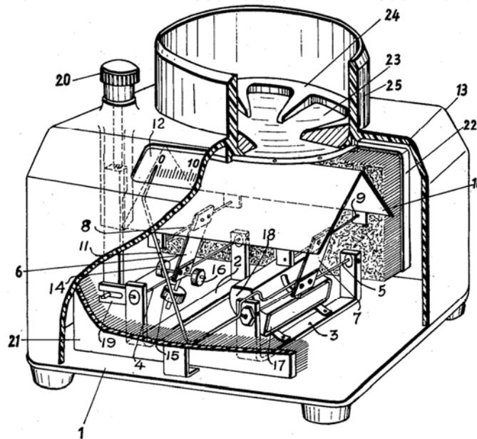
Fig 9. Cutaway plan of the Fiedler portable power balance as shown in the patent. Hueter & Bolt [18].
