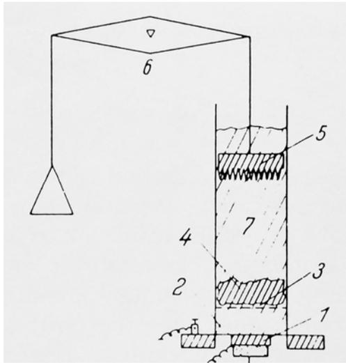
Fig 7. Pohlman's use of radiation force to measure ultrasound transmission loss in samples of tissue. 1 & 2 quartz fixed to tin foil: 3 & 4 tissue sample laid on a paper sheet: 5 scattering target: 6 arm of a sensitive balance: 7 sodium chloride solution. Pohlman, 1939. [17]
