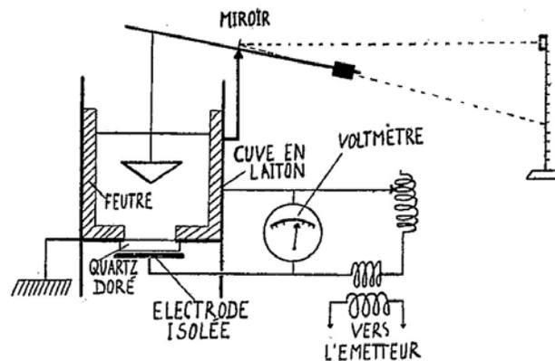
Figure 5. Ernest Baumgardt's balance with vertical beam and conical target. 1937. [13]
