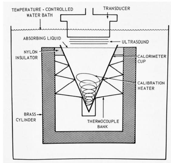
Fig 9. Stewart's steady-state calorimeter for therapy power measurements. 1974. [24]
