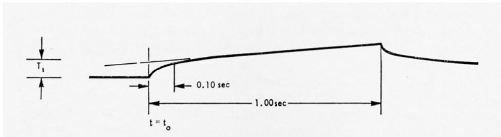
Fig 7. Temperature-time profile from Fry's thermocouple probe. (©Ilfiffe Books Ltd)
