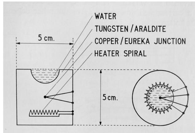
Fig 8. The Bristol ultrasonic calorimeter
