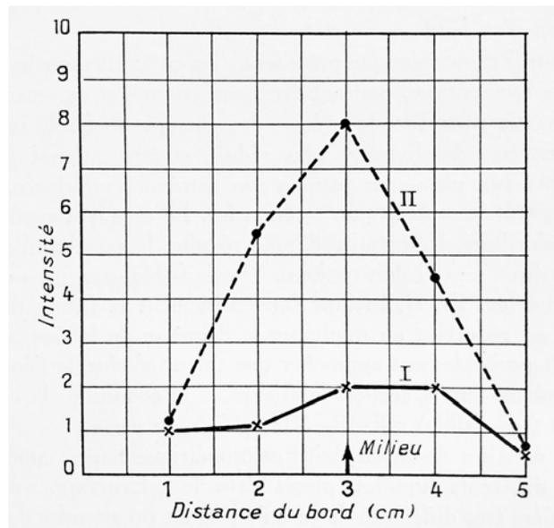
Fig 2. Relative intensity beam profile using a *tube calorimétrique*. [3]
