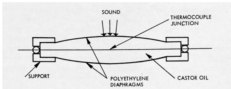
Fig 5. Intensity probe using a thermocouple in castor oil. Fry & Fry. 1954. [12] (©Iiffie Books Ltd)
