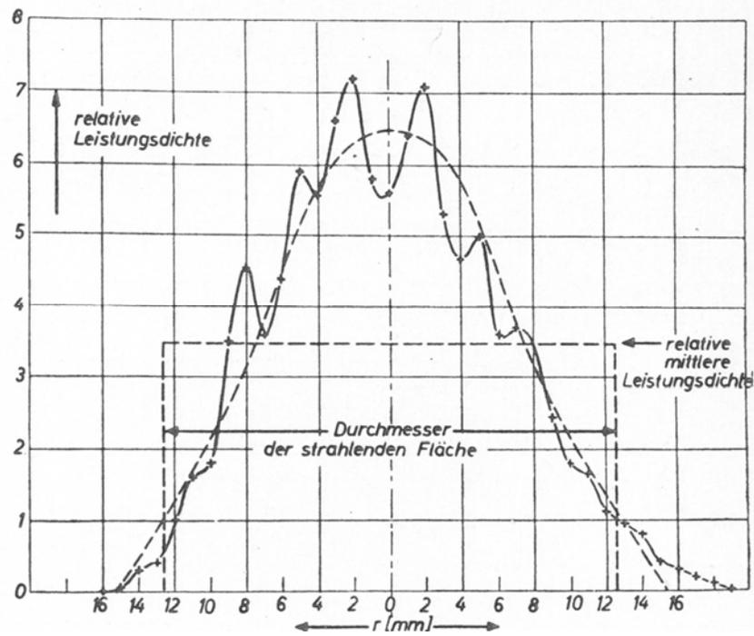
Fig 4. Near-field relative intensity profile (continuous line) in the near field of a 25 mm diameter transducer, measured using a thermal probe at PTB, Brunswick, 1952. The dashed curve was calculated assuming radial symmetry and omitting diffraction. [7]
