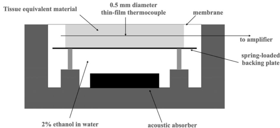
Fig 12. Thermal Test Object (redrawn). [49]
