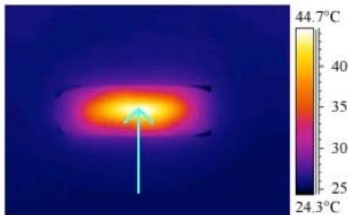
Fig 13. Thermal image of the front surface of an ultrasound array in Doppler mode, operating in air. The arrow identifies the point of maximum temperature rise. [57] (British Medical Ultrasound Society)
