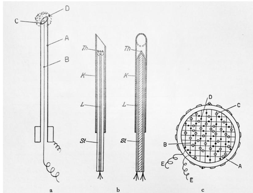
Fig 3. Pohlman's thermocouple probes, 1950 [5].
