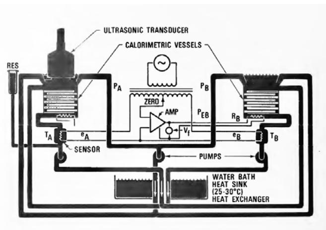
Fig 10. The NBS two-chamber servo-controlled calorimeter 1976. [31] (Reprinted courtesy of the National Institute of Standards and Technology, U.S. Department of Commerce).
