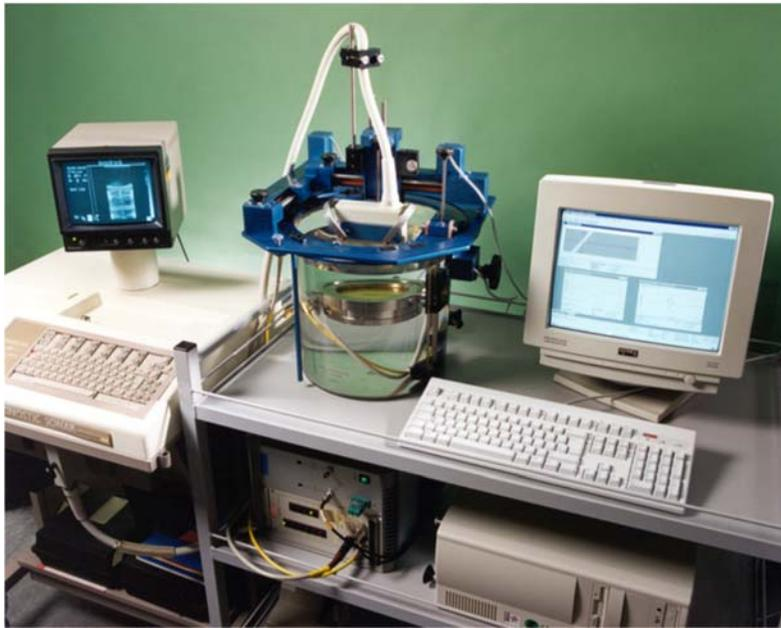
Fig. 15 The NPL Ultrasound Beam Calibrator. (Image courtesy of Dr B Zeqiri, NPL, Teddington, UK)
