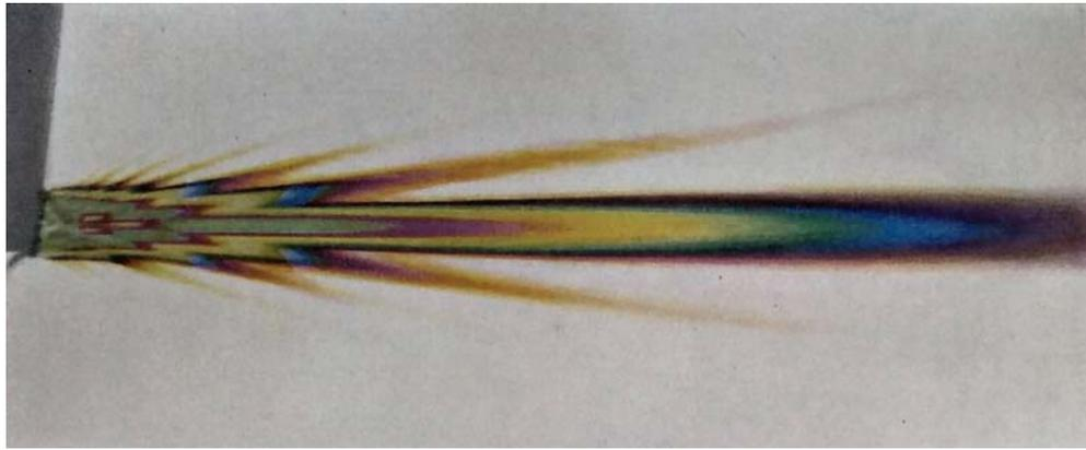
Fig 9. Beam from a source,  $11 \lambda$  diameter, in  $C_6H_6$ , Hiedemann & Osterhammel 1938 [33].
