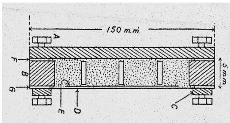
Fig 2. Experimental large area carbon hydrophone. Langevin 1917. The carbon granules are packed in water between a brass disc A and a sheet of mica D, clamped onto an ebony ring B. A steel plate E is cemented inside the mica. Glass panels prevent the carbon becoming too tightly packed.
