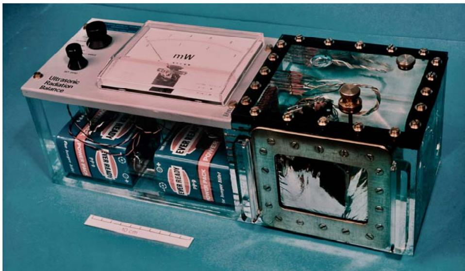
Fig 17. Farmery and Whittingham portable milliwatt power balance [45]
