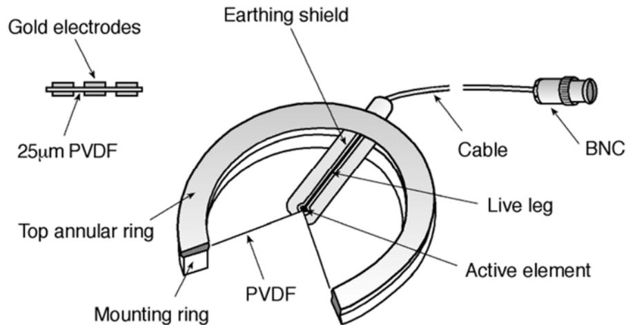
Fig. 7 The electrode configuration of the coplanar shielded membrane hydrophone. (Image courtesy of Dr B Zeqiri, NPL, Teddington, UK)
