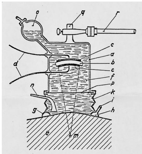
Fig 15. Siemens patented focused bowl transducer for treatment. 1935. [77].
