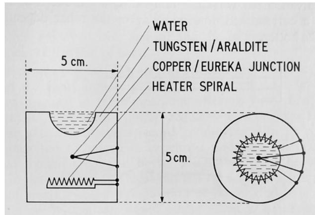
Fig 8. The Bristol ultrasonic calorimeter
