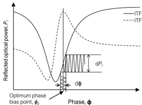
Fig. 18 The intensity-phase transfer functions (ITF) for a Fabry-Pérot interferometer. (Reprinted with permission from Morris P, Hurrell A, Shaw A, Zhang E, Beard P. A Fabry-Pérot fiber-optic ultrasonic hydrophone for the simultaneous measurement of temperature and acoustic pressure. *J Acoust Soc Am* 2009; 125: 3611–3622. Copyright 2009, Acoustic Society of America.)
