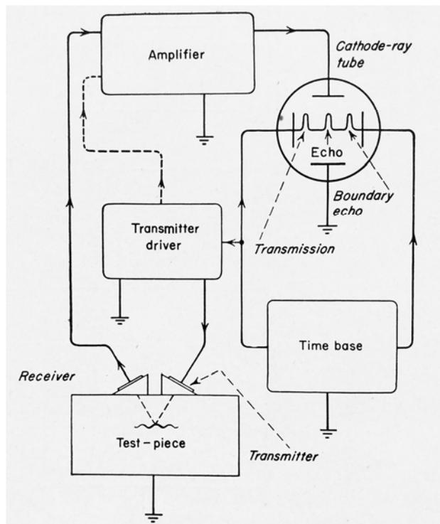
Fig 22. Block diagram from the Hughes pulse-echo system. 1943.
