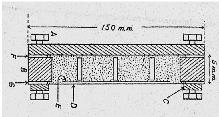
Fig 2. Experimental large area carbon hydrophone. Langevin 1917. The carbon granules are packed in water between a brass disc A and a sheet of mica D, clamped onto an ebony ring B. A steel plate E is cemented inside the mica. Glass panels prevent the carbon becoming too tightly packed.
