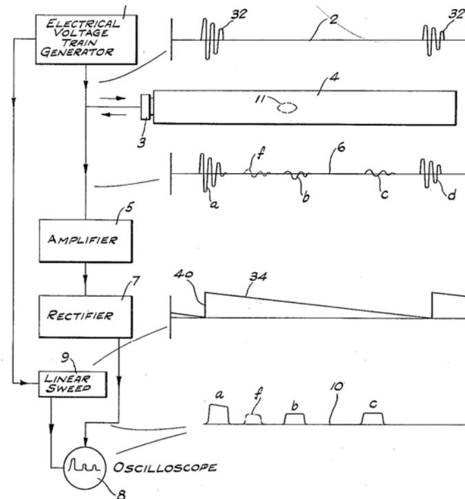
Fig 21. Block diagram from Firestone's pulse-echo patent. 1942
