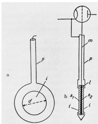
Fig. 1 Langevin's quartz crystal probe (1926). a) Front view. b) cross section.  $k_1$   $k_2$  quartz plates;  $l$  metal plate;  $p$  metallic housing;  $m$  insulated cable;  $i$  electrodes. (From Langevin 1926) [1]
