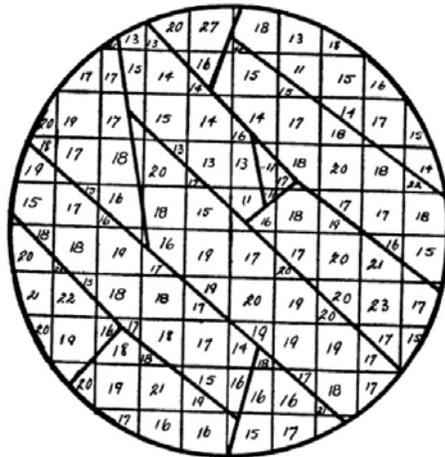
Fig 5. A quartz mosaic marked with the relative sensitivities of each element. (Boyle, [31])
