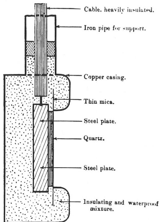
Fig 7. Boyle's broad-band encapsulated asdic transducer.
