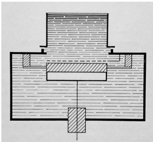
Fig 13. The French SCAM physiotherapy transducer (c.1933).
