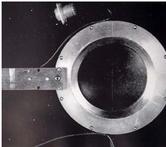
Fig 6. Beam's eye view of the Fry thermal probe.
