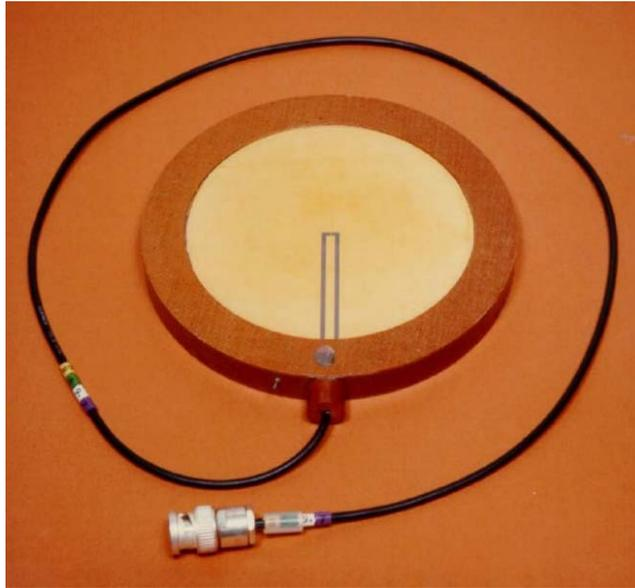
Fig. 6 An early NPL/Marconi bilaminar membrane hydrophone. (Image courtesy of Dr B Zeqiri, NPL, Teddington, UK)
