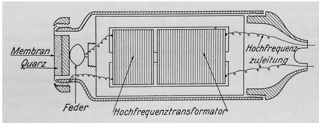
Fig 16. Ultrasound transducer for therapy. 800 kHz. Pohlmann 1939.
