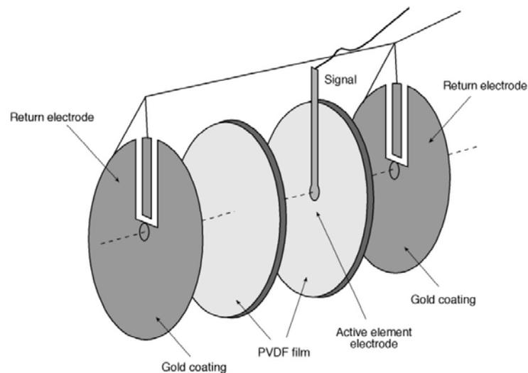
Fig. 8 Construction of the bilaminar shielded membrane hydrophone. (Image courtesy of Dr B Zeqiri, NPL, Teddington, UK)
