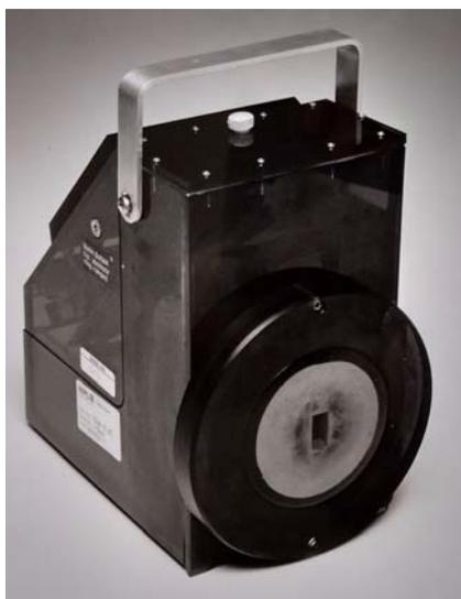
Fig 19. The Perkins ‘Bath’ Balance fitted with a 1 cm aperture for measurements for Thermal Index for scanned beams.
