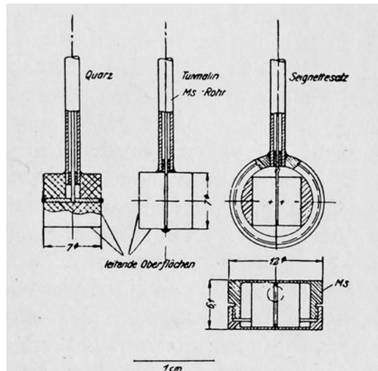
Fig. 2 Three alternative hydrophones, using quartz, tourmaline and Rochelle (Seignette) Salt. (From Meyer and Tamm 1939) [5]
