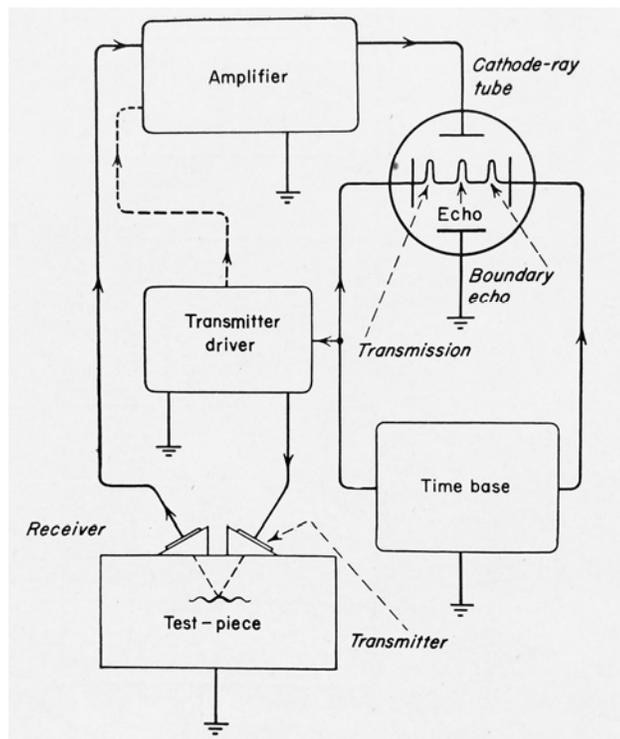
Fig 22. Block diagram from the Hughes pulse-echo system. 1943.
