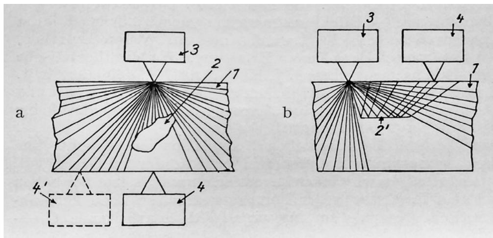
Fig 19. Ultrasonic materials testing by transmission (a) and reflection (b). 3: transmitter: 4,4': receiver. Mühlhäuser 1931. [94]
