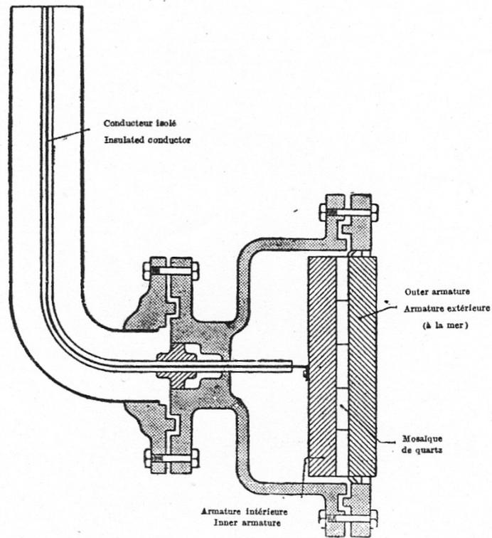
Fig 6. The Langevin-Florrison resonant quartz sandwich transducer.
