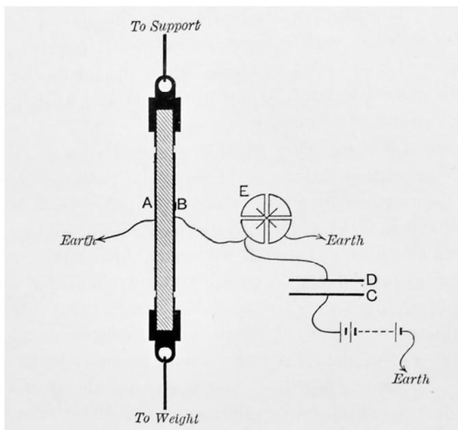
Fig 3. The quartz piézo-électrique for measurement of ionization. Piezoelectric charge across the quartz AB is balanced against the capacitor charge CD using the electrometer E, radioactivity measured by the discharge time for a fixed weight. Rutherford *Radioactivity* (1904).
