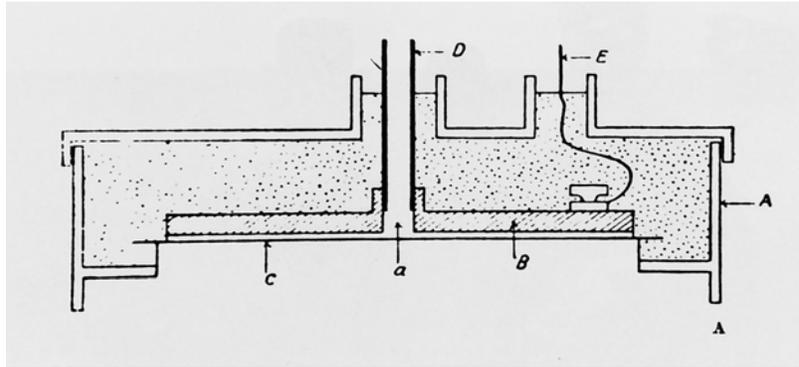
Fig 1. Langevin's singing condenser transducer c. 1916, consisting of a circular metal disc (B), mica sheet (C), vacuum tube (D) and box (A) filled with insulating compound.
