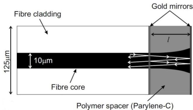
Fig. 17 The sensor head of a Fabry-Pérot miniature optical fibre hydrophone. (Reprinted with permission from Morris P, Hurrell A, Shaw A, Zhang E, Beard P. A Fabry-Pérot fiber-optic ultrasonic hydrophone for the simultaneous measurement of temperature and acoustic pressure. *J Acoust Soc Am* 2009; 125: 3611–3622. Copyright 2009, Acoustic Society of America.)
