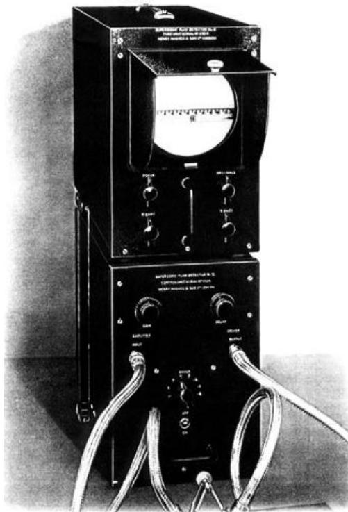
Fig. 1 The Kelvin and Hughes Mark IIb Flaw Detector.
