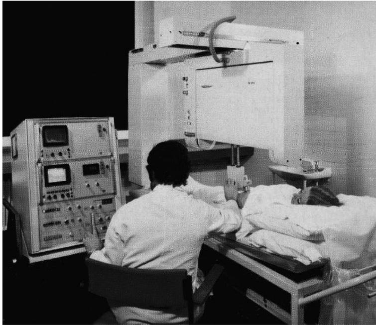
Fig.22. The NE 4102 Disonograph. From Bulletin No. 64 - New Disonograph NE4102 Diagnostic Ultrasonic Scanner. Nuclear Enterprises Ltd, 1972 [60].
