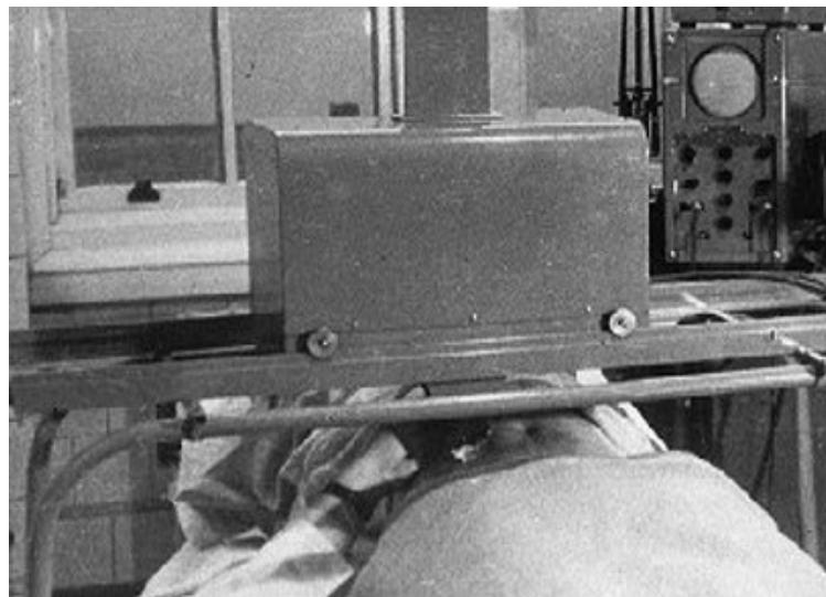
Fig. 7 Tom Brown’s bed-table scanner, c 1957. Note the restricted room for the operator’s forearm and hand (seen lower left). Photo courtesy of the BMUS Historical Collection
