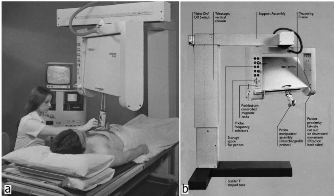
Fig. 26 a) The EMISONIC 4200 Disonograph. b) Annotated image of the mechanical system. From Nuclear Enterprises Bulletin No. 112 (1977) [70].
