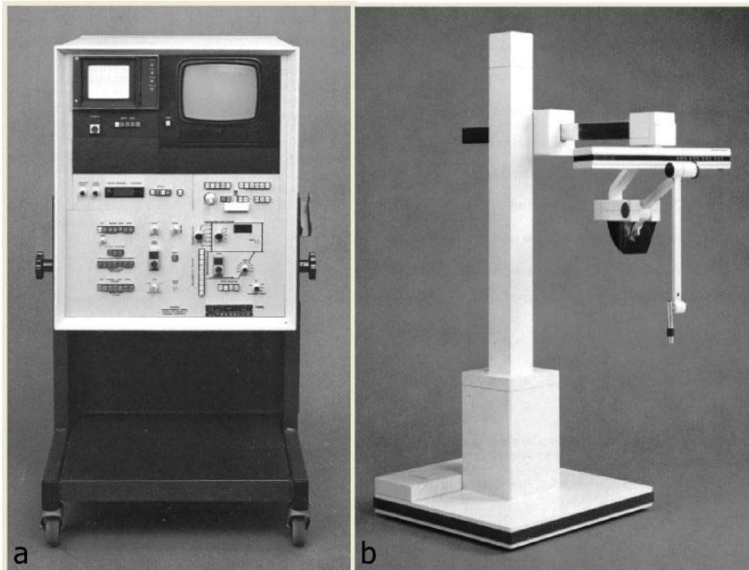
Fig. 29 a) Fischer 4200S console. From Fischer Ultrasound sales leaflet for 4200S [74]. b) Articulated arm option for the Fischer 4200S. From Fischer Ultrasound sales leaflet for the Articulated Scan Arm [76].
