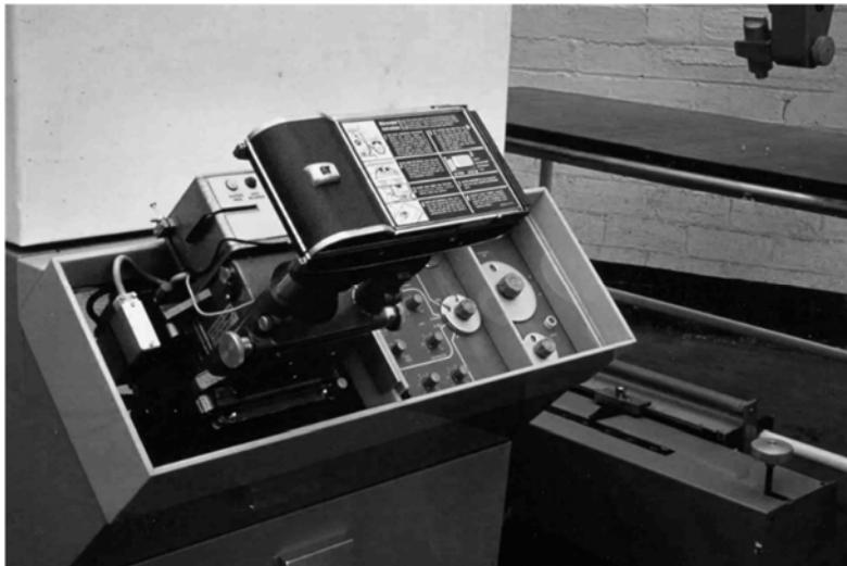
Figure 21. The controls on the console of the Smiths' Diasonograph, with the three levels of control and Polaroid camera, designed by Dugald Cameron. Photo reproduced by the kind permission of Dugald Cameron
