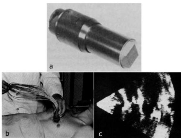
Fig. 36 a) Phased array probe made by Jan Somer of Utrecht University in 1968. Courtesy of Jan Somer. b) Prototype phased array from Frederick Thurstone's group at Duke University. c) Example of a heart scan from the Duke University. Photos b) and c) reproduced from Kisslo et al (1976) [93].
