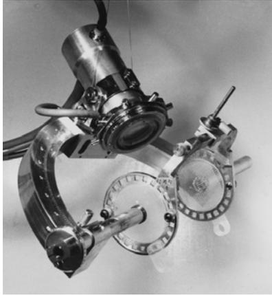
Fig. 4 Transducer head and stereotactic frame developed by Lindstrom & Leksell. (photo courtesy of Dan Leksell)
