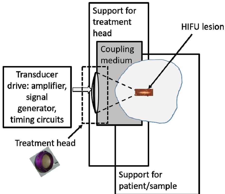
Fig 2. Schematic showing the necessary components of a HIFU system.
