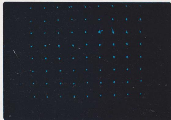
Cross-sectional picture of a matrix of wires spaced at 0.5in (12.7mm) intervals in a water tank
