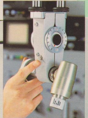
Finger tip two-directional control of stepping motor.
