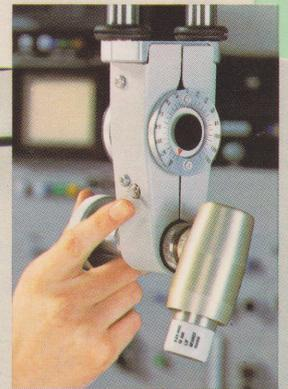
Finger tip two-directional control of stepping motor.
