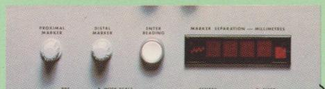
0.1% accurate digital caliper. Pushbutton readout onto display.
