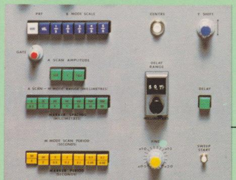
Pushbutton automatic centering of image, colour coded controls of 'B' Scan, 'A' Scan and 'M' mode operations.
