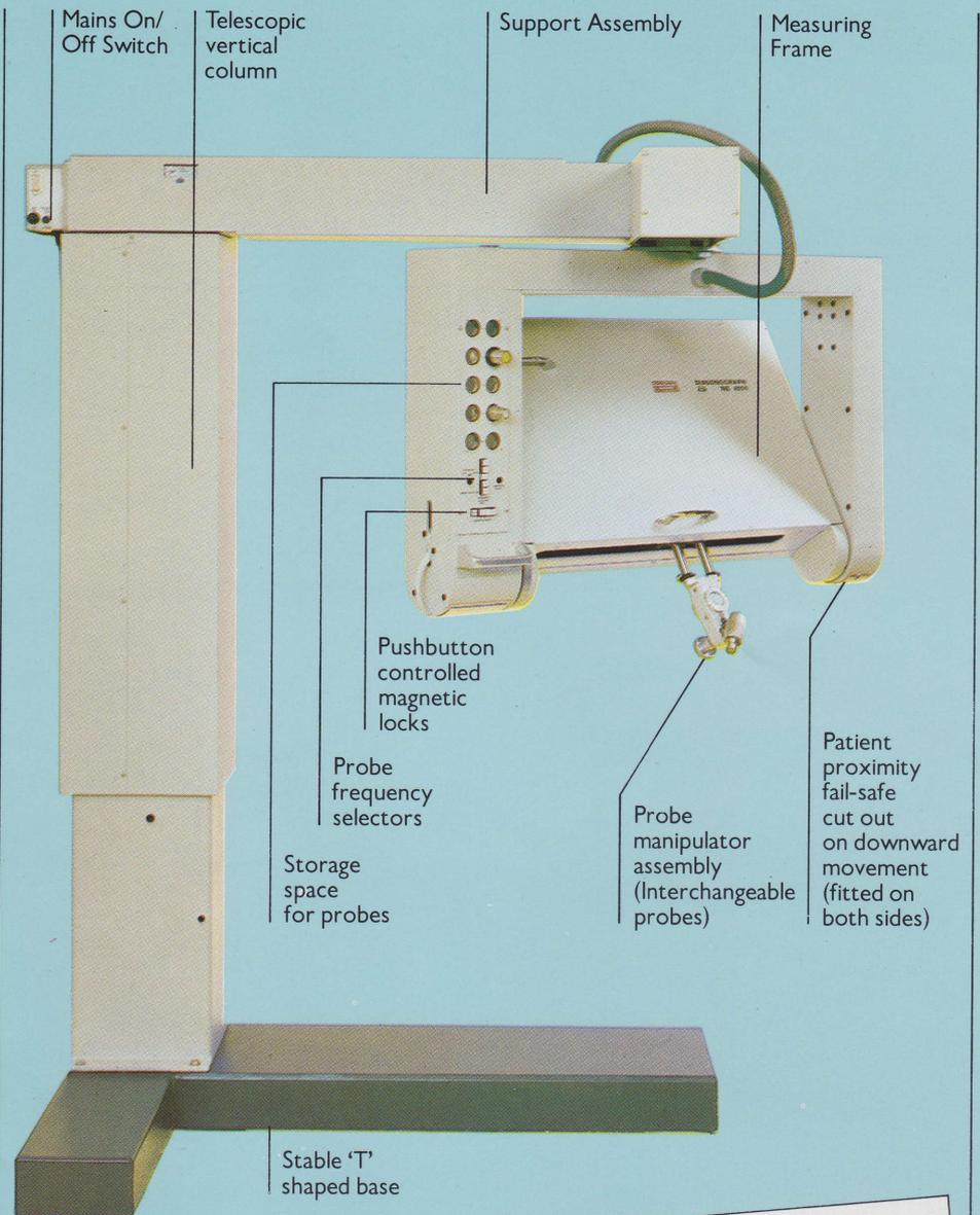
The ultrasonic power output in all Nuclear Enterprises scanners is reduced to the lowest possible level in order to minimise the dose energy to the patient, whilst maximising the use of it. The sensitivity of the equipment is controlled by reducing the transmitted power rather than using high power and reducing the gain of the system.
