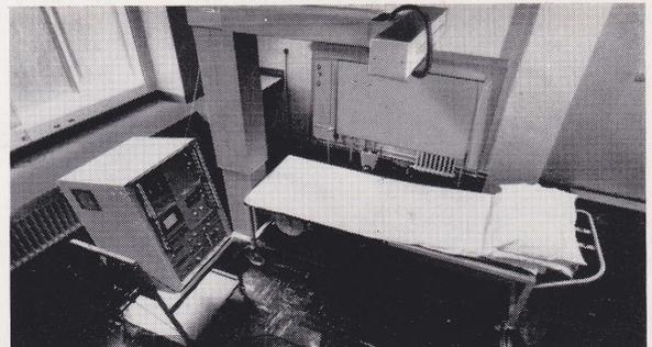
In the new Disonograph, maximum use has been made of floor space without any scuffing in the facility of selecting the more difficult scanning planes. The construction of the scanning system and the control cabinet affords considerable freedom of choice in the layout of the examination room. Total system weight is 650kg. (Photo courtesy Design Magazine and Philip Sayer)
