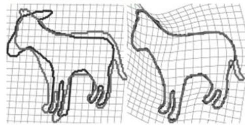
Fig 4 Deformable image registration (DIR) is the process of registering an image data set to a reference image data set by applying an elastic deformation to minimise the difference between the two. This allows comparison or integration of data which is obtained from two different measurements –from the ‘Deformable Image Registration (DIR)’ article
