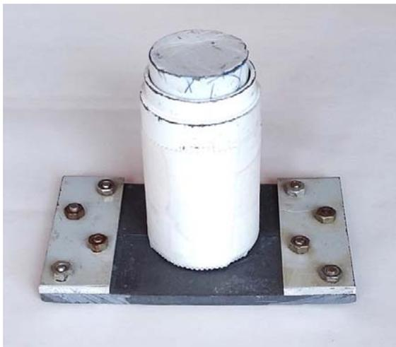
Fig. 1 Slit phantom with encapsulated source.
