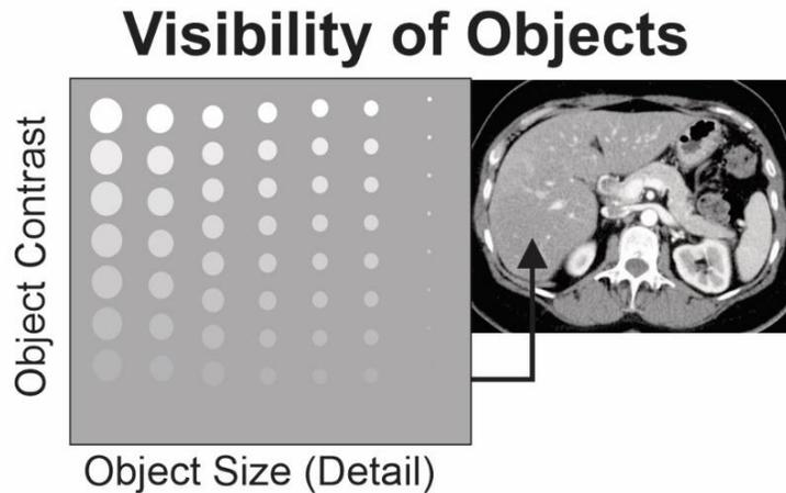
Figure 28. A Contrast Detail test device or phantom (shown on the left) contains objects with varying contrast and size/detail to represent the range of objects in the human body.
