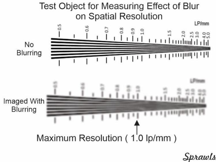
Figure 30. A test device with varying spatial resolution (size and distance between opaque lines) expressed in line pairs (a line and a space) per millimeter (mm) of distance.
