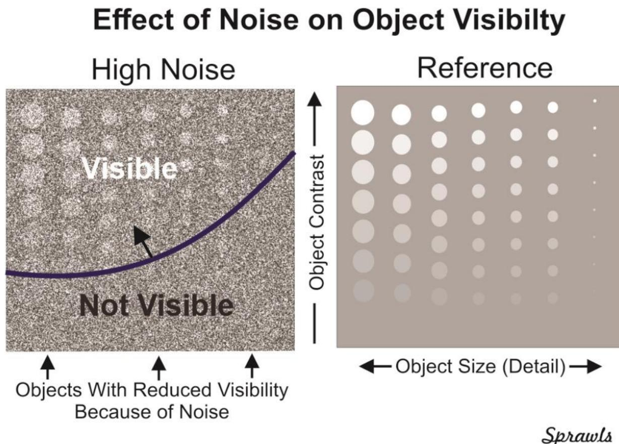
Figure 27. Illustrating image characteristics by processing an image (Reference) with a pixel-based Paint program
