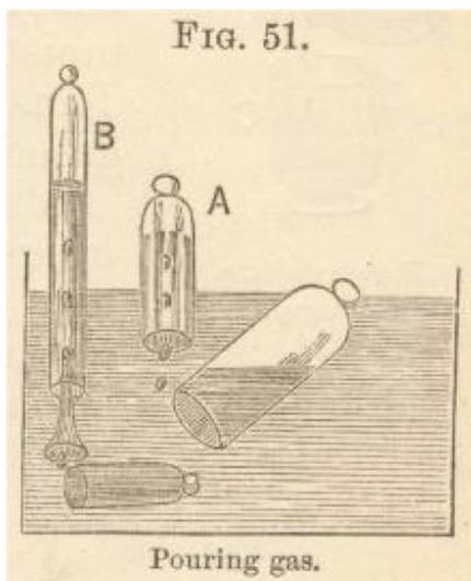
It is generally easy to pour a liquid from one container to another with the help of gravity. How do you pour a gas? One method used in the physics laboratory is illustrated here. It is done in a large container of water. An empty container, with respect to gas, is filled with water and with the opening down in the larger water container. When a gas is poured from another container it displaces the water as it bubbles up into the receiving container.
