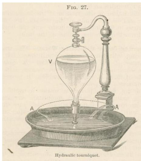
One of the principles of hydrodynamics, or fluid in motion, is demonstrated in Fig. 27. Specifically, that forces are created by moving fluid. The hydrostatic pressure in the glass container forces water out through the small openings at the end of the tubes.
