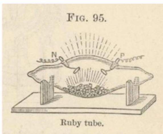
Shown here in Fig. 95 is the Ruby Tube developed by Professor Crookes. Various substances are placed in the highly evacuated (about one millionth of an atmosphere). When the electrodes are connected to a coil providing a high voltage the
