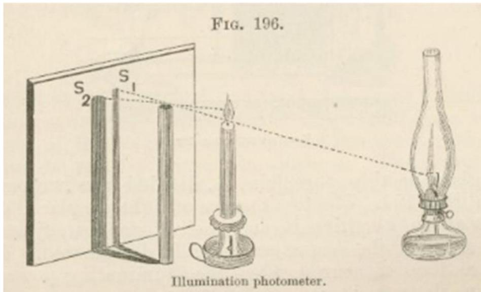
*Rumford's photometer* illustrated in Fig. 196 was one method used to measure the intensity of a light source. An opaque rod is located a short distance in front of a screen as shown. The two light sources that are to be compared are moved until their shadows appear with the same intensity. The intensity of each is proportional to the square of the distance between the light source and screen.
