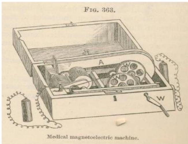
The principle of magnetic induced currents was used to explain the operation of the “magnetolectric” machine shown in Fig. 363. It contains a large horse-shoe magnet (A) and a mechanism for rotating a small metal object between the magnetic poles. As the magnetism in the object fluctuates with the rotation, an electric current is induced in a coil around the rotating object. The machine was used to pass electrical currents through the human body for medical purposes.
