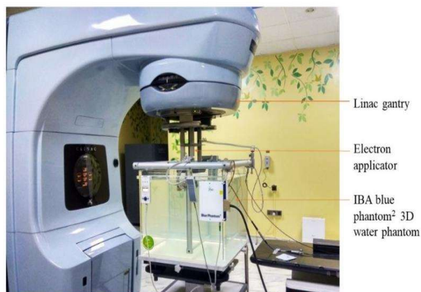
Figure 2. Experimental set-up for obtaining electron beam depth-dose distributions
