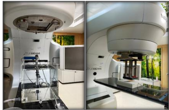
Fig. 2: Set-up and images for monthly QA
